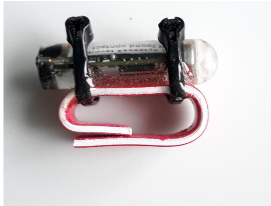
Figure 5. Cefas G5 Time Depth Recorder tag (TDR) mounted on a 2mm red darvic ring, specially shaped for fitting to a red-throated diver's tarsus. Photo: Sue O'Brien.
