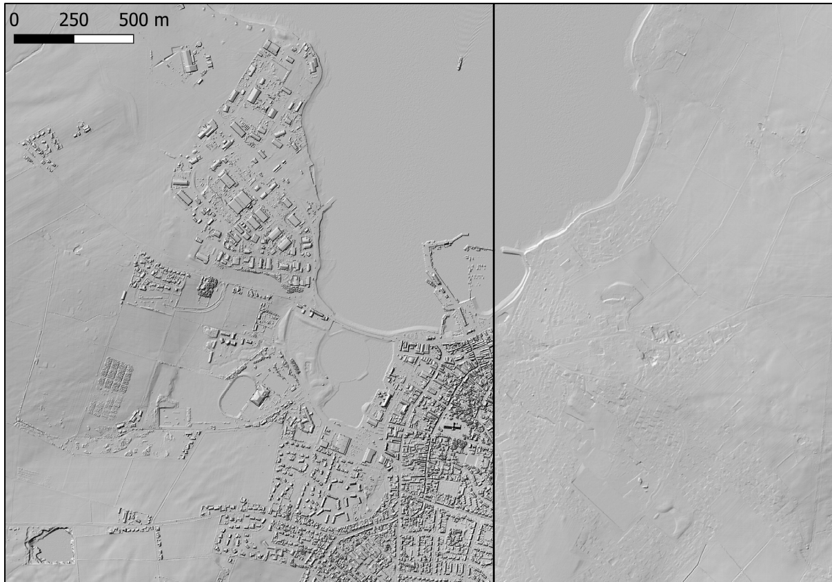
Figure 7. 1m resolution LiDAR DSM (left) and DTM (right) of Kirkwall, Orkney. Data from the Scottish Remote Sensing Portal [accessed June 2020]. A hillshade visualisation has been applied in QGIS.
