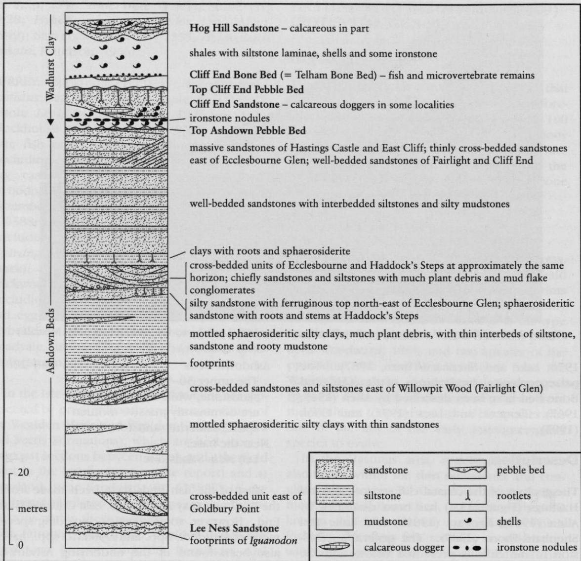
**Figure 13.5** Stratigraphical log of Cliff End section, near Hastings (after Lake *et al.*, 1987).
