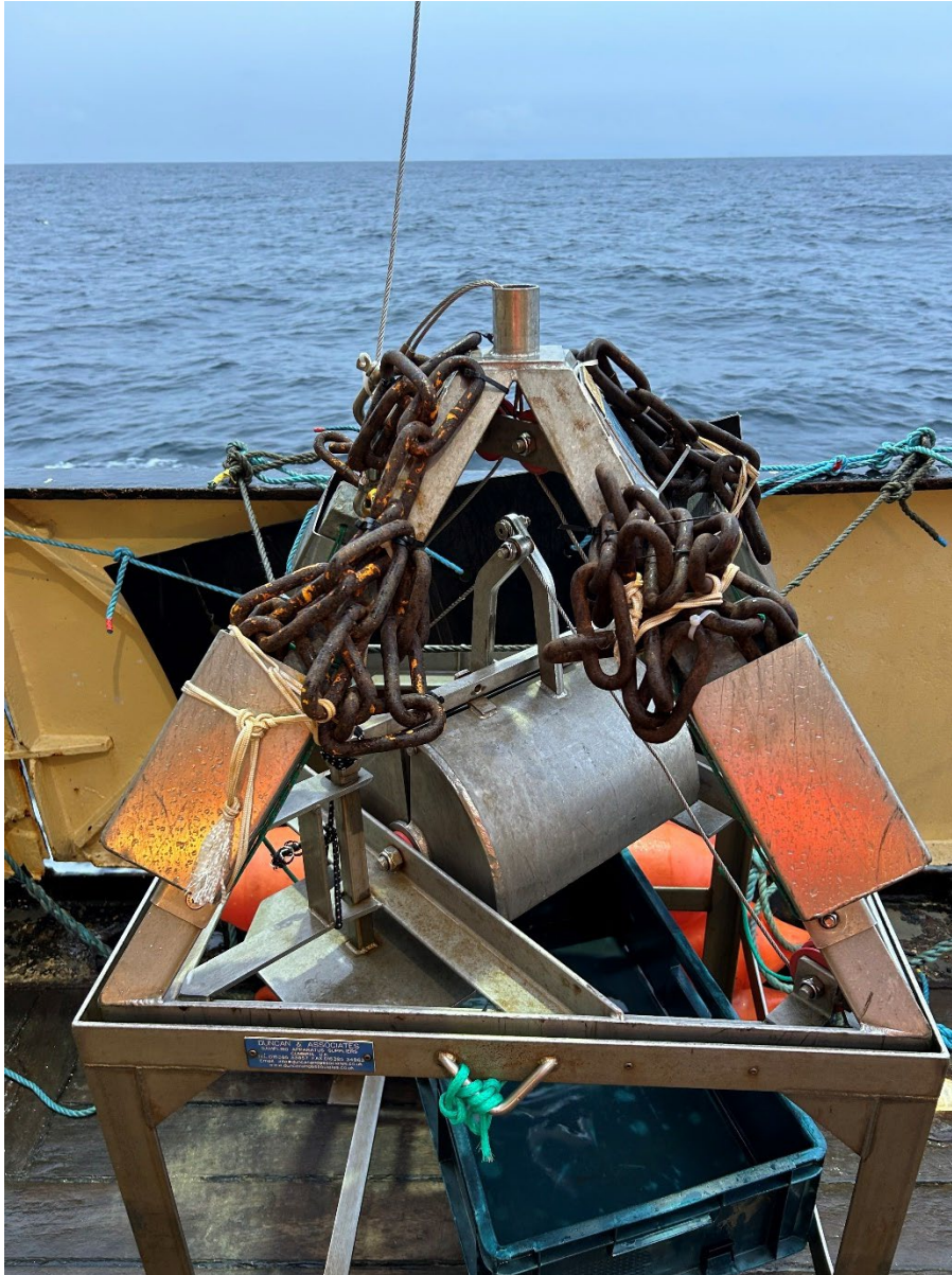
Figure 8. 0.1 m 2 Day grab used on the COR0924 mNCEA survey. Chain was added for extra weight in absence of lead.
