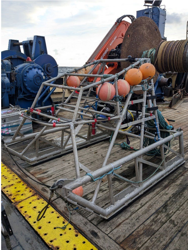
Figure 9. Camera sledge frame used on COR0924 mNCEA survey.
