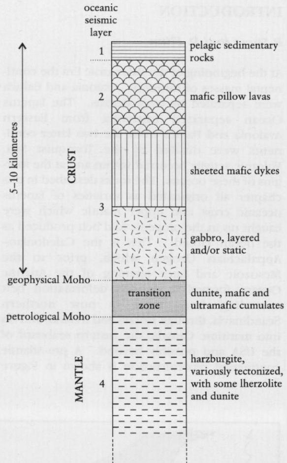
**Figure 2.2** An idealized ophiolite succession compared to the seismic structure of oceanic crust and mantle (after Coleman, 1977). As an indication of scale, beneath the oceans the depth to the geophysical moho is between 5 and 10 km.
