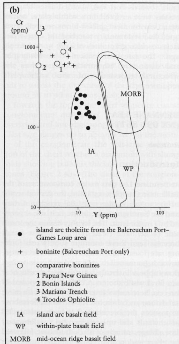
**Figure 2.38** Geochemical discrimination diagrams for Ballantrae Complex basalt lavas: (a) Ti-Zr-Y, fields from Pearce and Cann (1973). (b) Cr-Y, showing comparison with representative boninites after Smellie and Stone (1992); fields from Pearce (1982).
