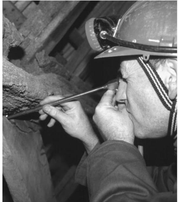
Bat worker using fiberscope to inspect mortice joints in barn.
