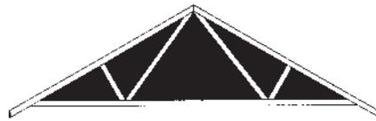
Trusses are prefabricated with metal plates at the joints
