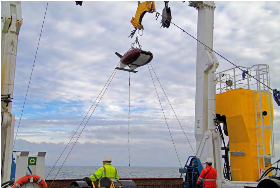
Figure 8. The Geoforce deep-towed boomer towfish being deployed from the RV Cefas Endeavour . The hydrophone streamer can be seen hanging from the rear of the towfish (Photo: Alan Judd, 2015).
