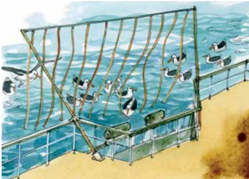
Figure 3. The Bird Exclusion Device or 'Brickle Curtain' is a deterrent that forms a protective barrier around the hauling hatch 6 .
