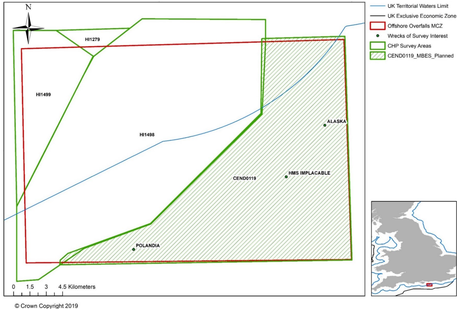
Figure 4. Map showing the areas where the MCA has collected MBES at OOVr and the remaining area to be surveyed during CEND0119. The locations of the three wrecks of interest identified by Historic England are also shown. Contains public sector information licensed under the Open Government Licence v3.0. Horizontal Datum WGS84, Projection – UTM Zone 30 N.
