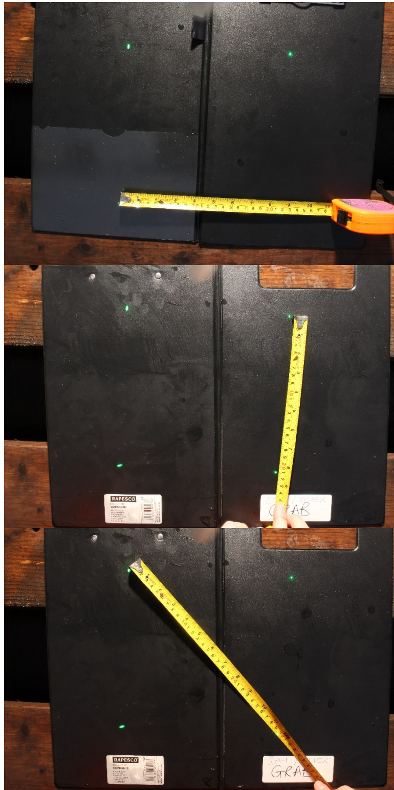
Figure 17. Four-spot laser-scaling (green) forming a 21cm x 21cm square. Diagonal measurement is 30cm.
