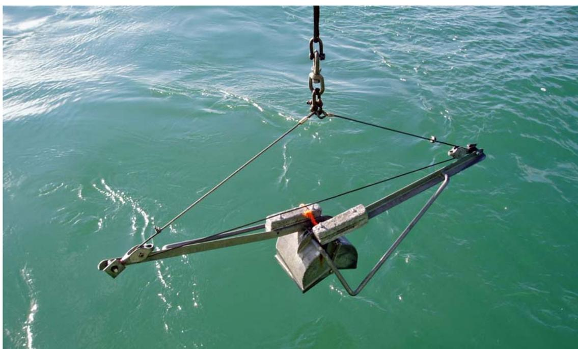
**Figure 6.** NMW Van Veen grab being deployed.
