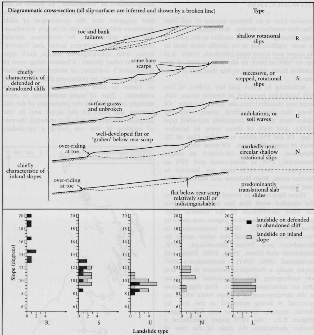
**Figure 8.2** Behaviour of London Clay cliffs following cessation of erosion at the toe. Cross-sections and slope-angle histograms illustrate the types of landslide found on slopes in London Clay as described by Hutchinson (1979).
