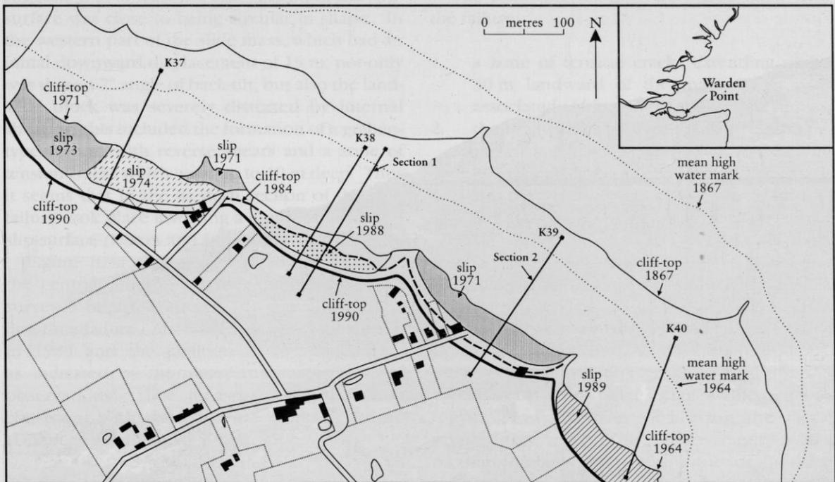
Figure 8.6 Landslides and location of cross-sections at Warden Point. Based on Hutchinson (1965) and Dixon and Bromhead (1991).
