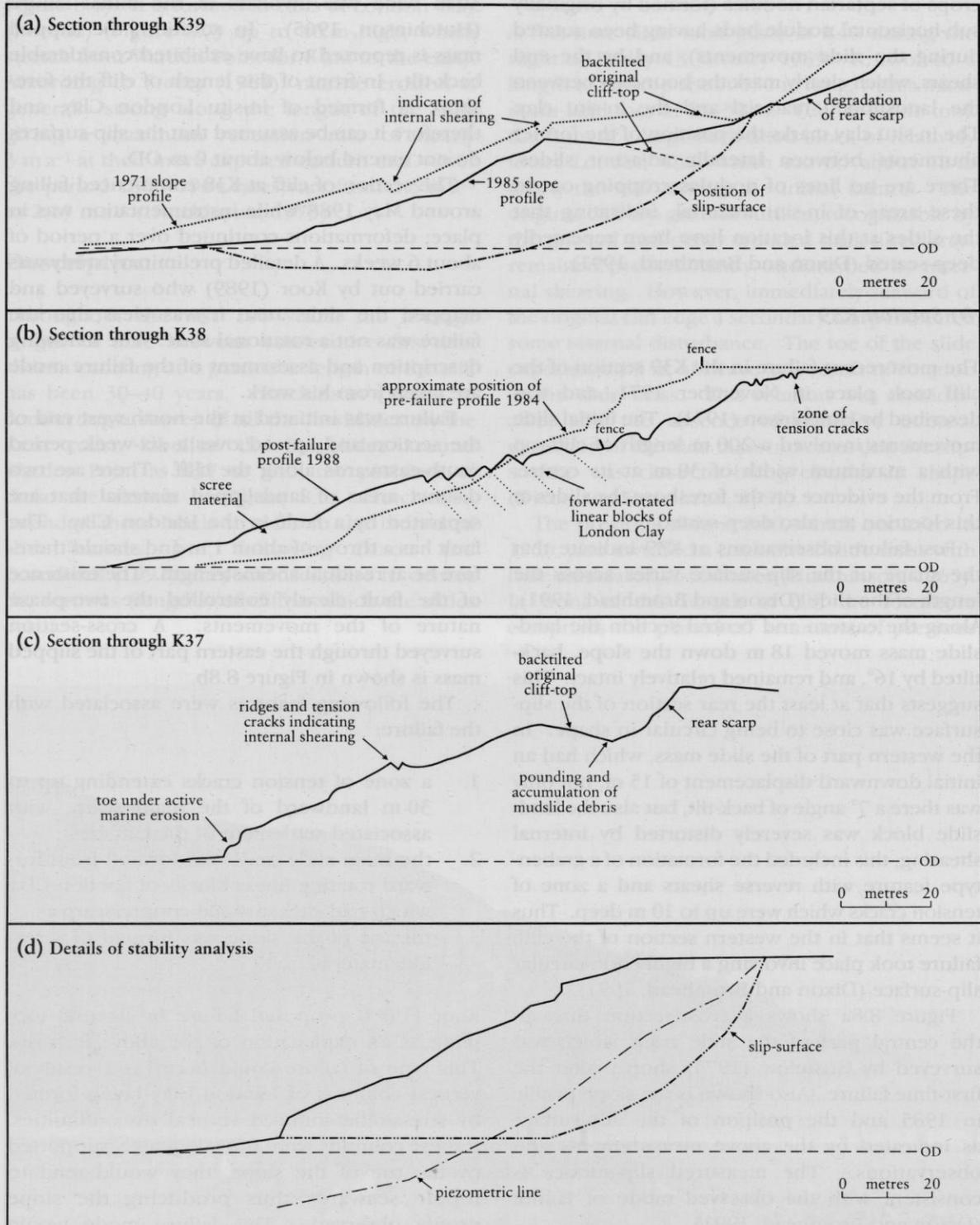
**Figure 8.8** Sections K37–9 (a–c) at Warden Point (after Lee, 1976; Koor, 1989; Dixon and Bromhead, 1991), and (d) K38 ‘idealized’ profile and slip-surface (after Bromhead and Dixon, 1984). See Figure 8.6 for locations of sections.
