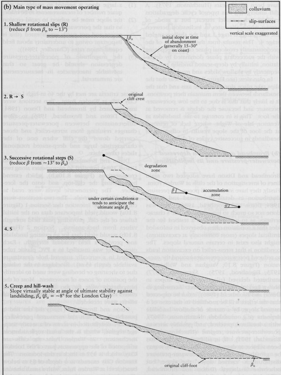
**Figure 8.9 – continued.** (b) Cyclic mechanism of mass movements in London Clay Cliffs, North Kent; for comparison with with Figure 8.9a. After Hutchinson (1967, 1970, 1973).
