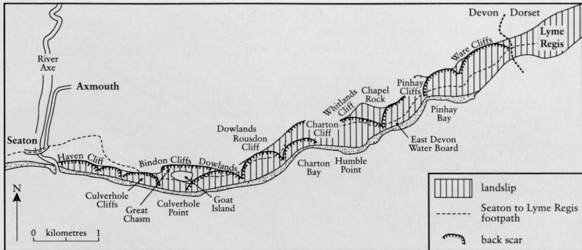
**Figure 6.20** The landslides of the Axmouth to Lyme Regis Undercliffs National Nature Reserve. After Pitts and Brunsden (1987).
