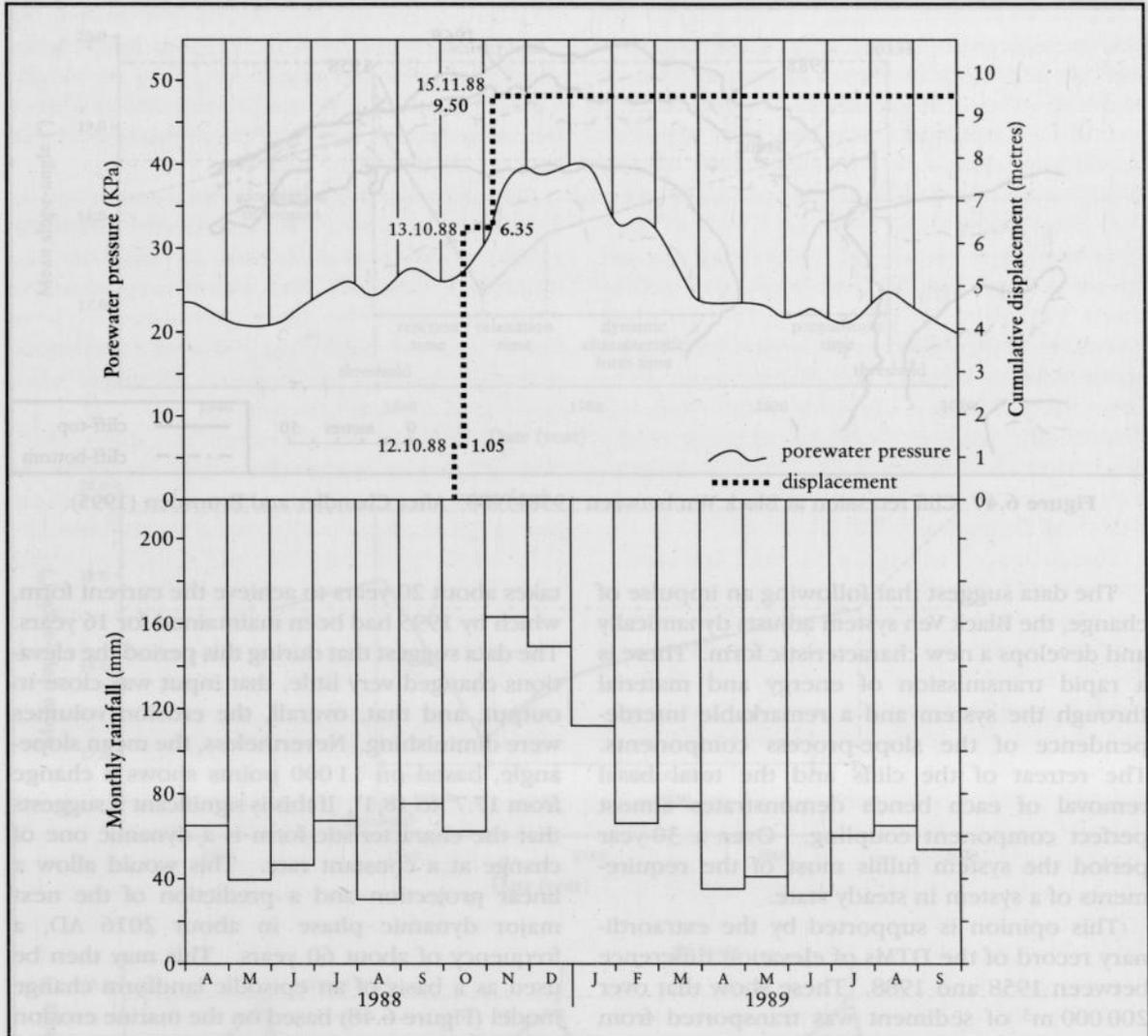
**Figure 6.46** The seasonal behaviour of rainfall movement and porewater pressure at Black Ven. The observation that movement ceased on 5/11/88 suggests that there may have been a considerable strength gain following movement. After Koh (1990).
