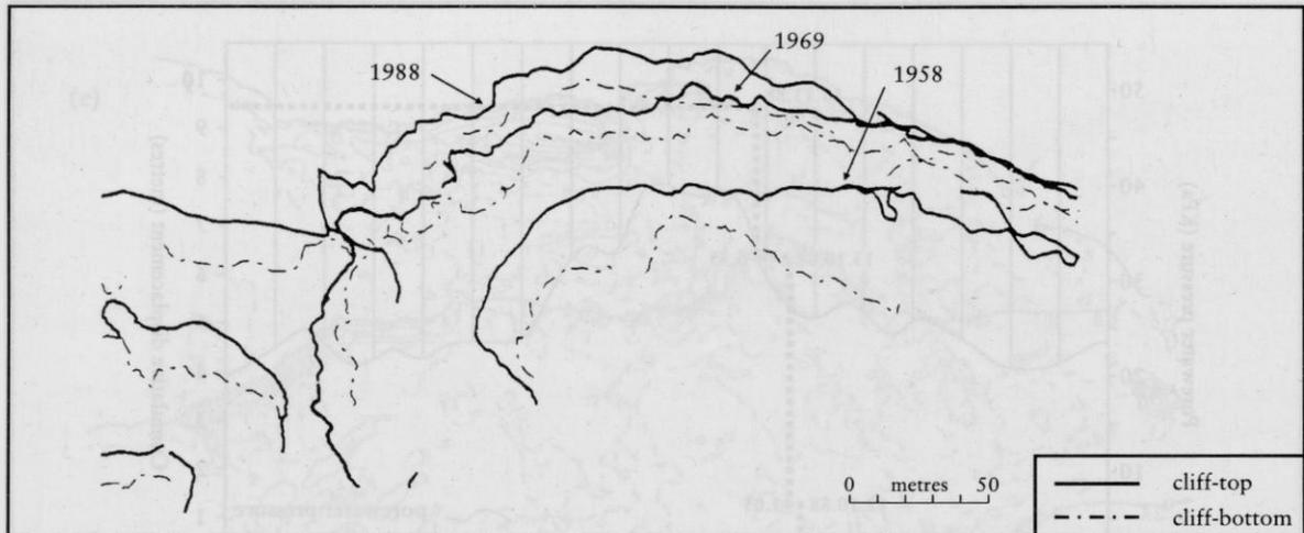
Figure 6.47 Cliff recession at Black Ven between 1958–1988. After Chandler and Brunsden (1995).
