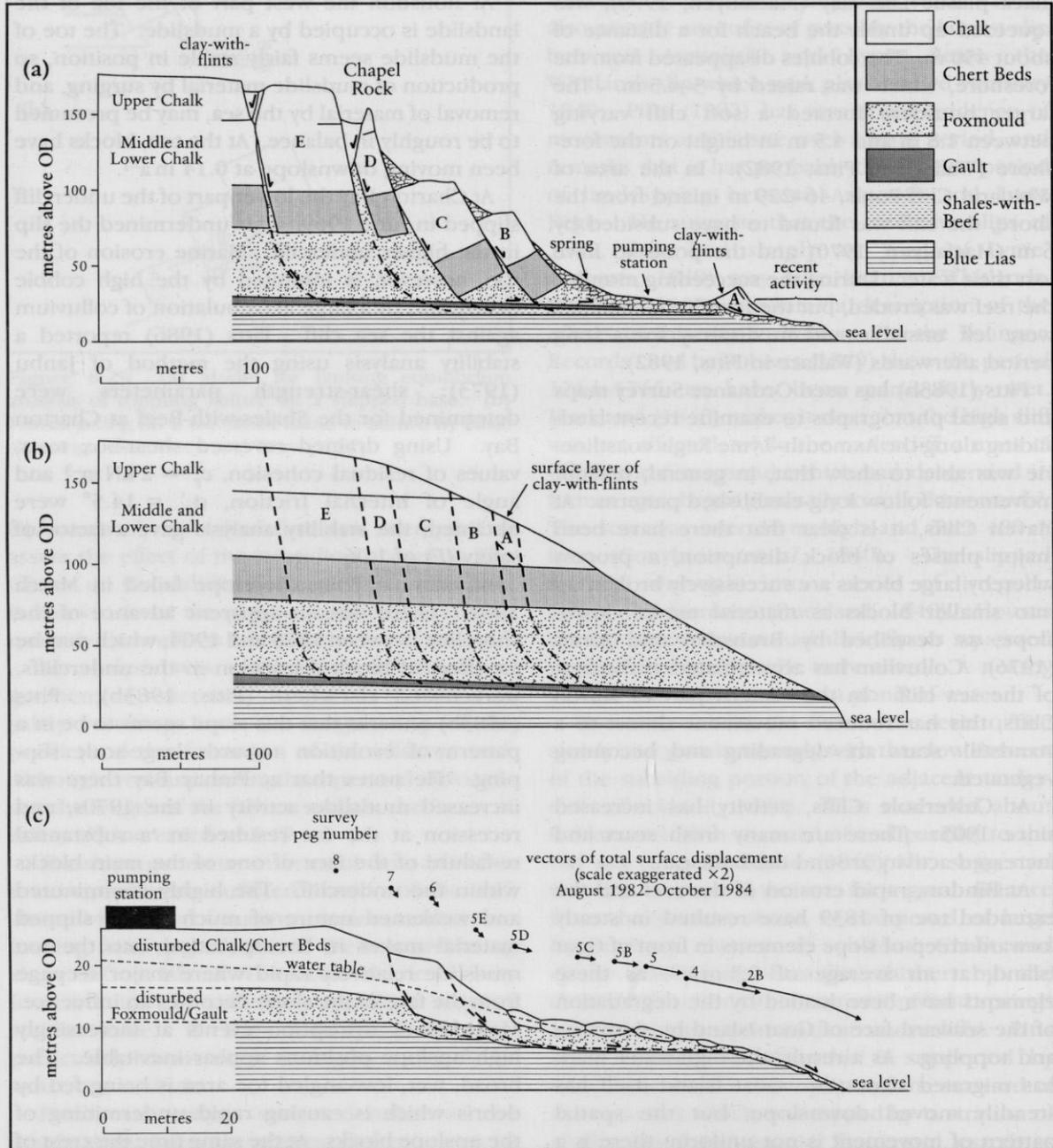
**Figure 6.30** Cross-sections and evolutionary reconstruction of the Chapel Rock landslide and the surveyed movements at the undercliff water pumping-station. Note the loss of the Foxmould by flow or extrusion. After Grainger *et al.* (1985).
