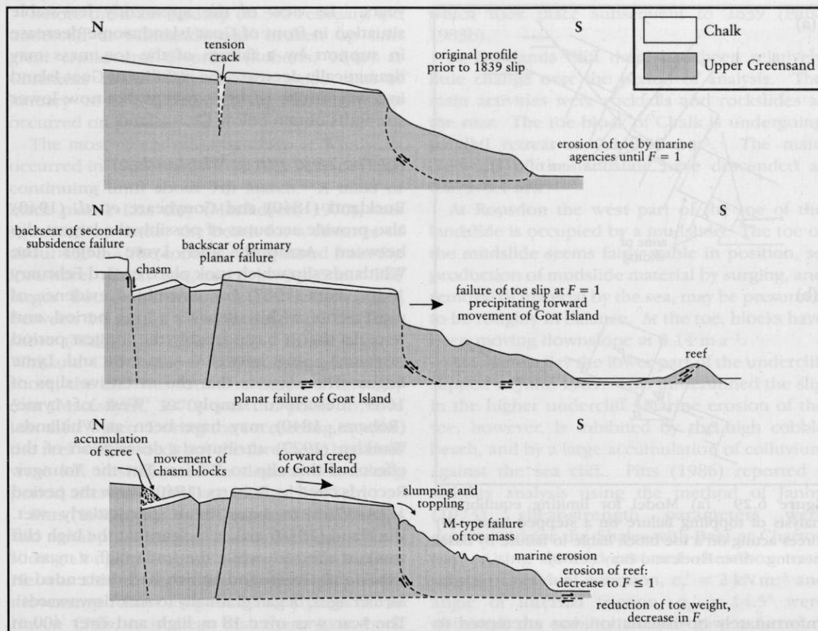
**Figure 6.28** Diagrammatic reconstruction of the development of the Bindon Landslide. ‘*F*’ refers to the factor of safety against landsliding. An M-type failure is a multi-rotational slide from the classification of Skempton and Hutchinson (1969). After Pitts and Brunsden (1987).
