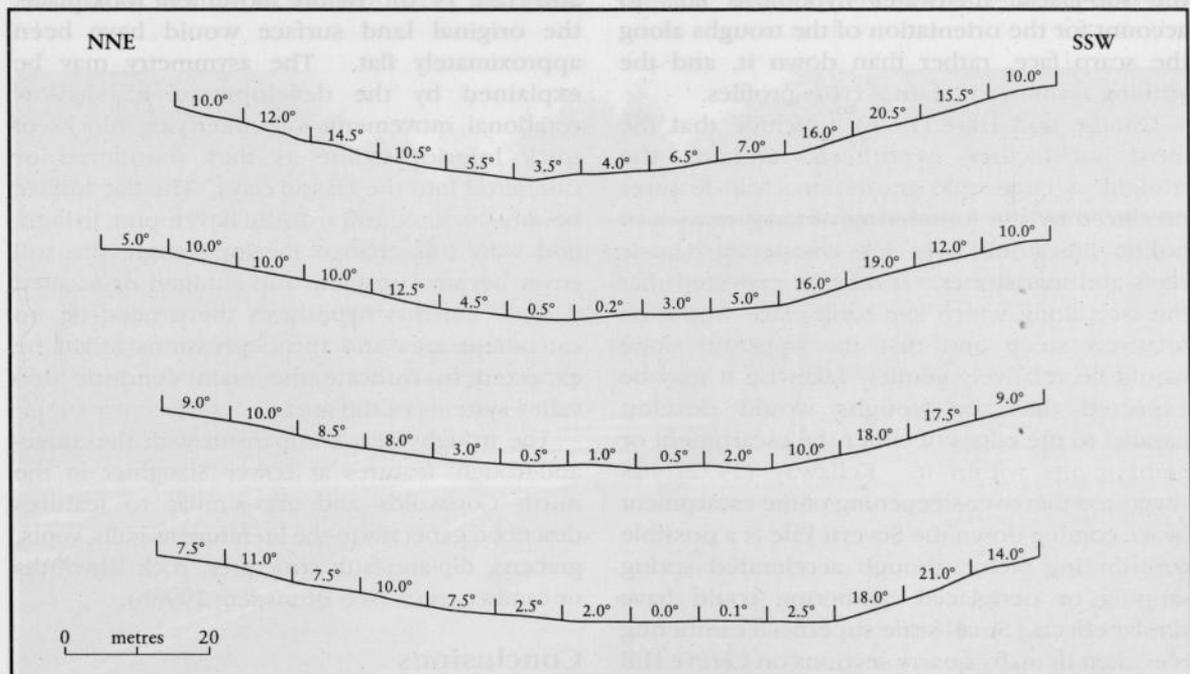
**Figure 6.4** Representative slope profiles at Postlip Warren to show distribution of maximum angles. After Goudie and Hart (1976).
