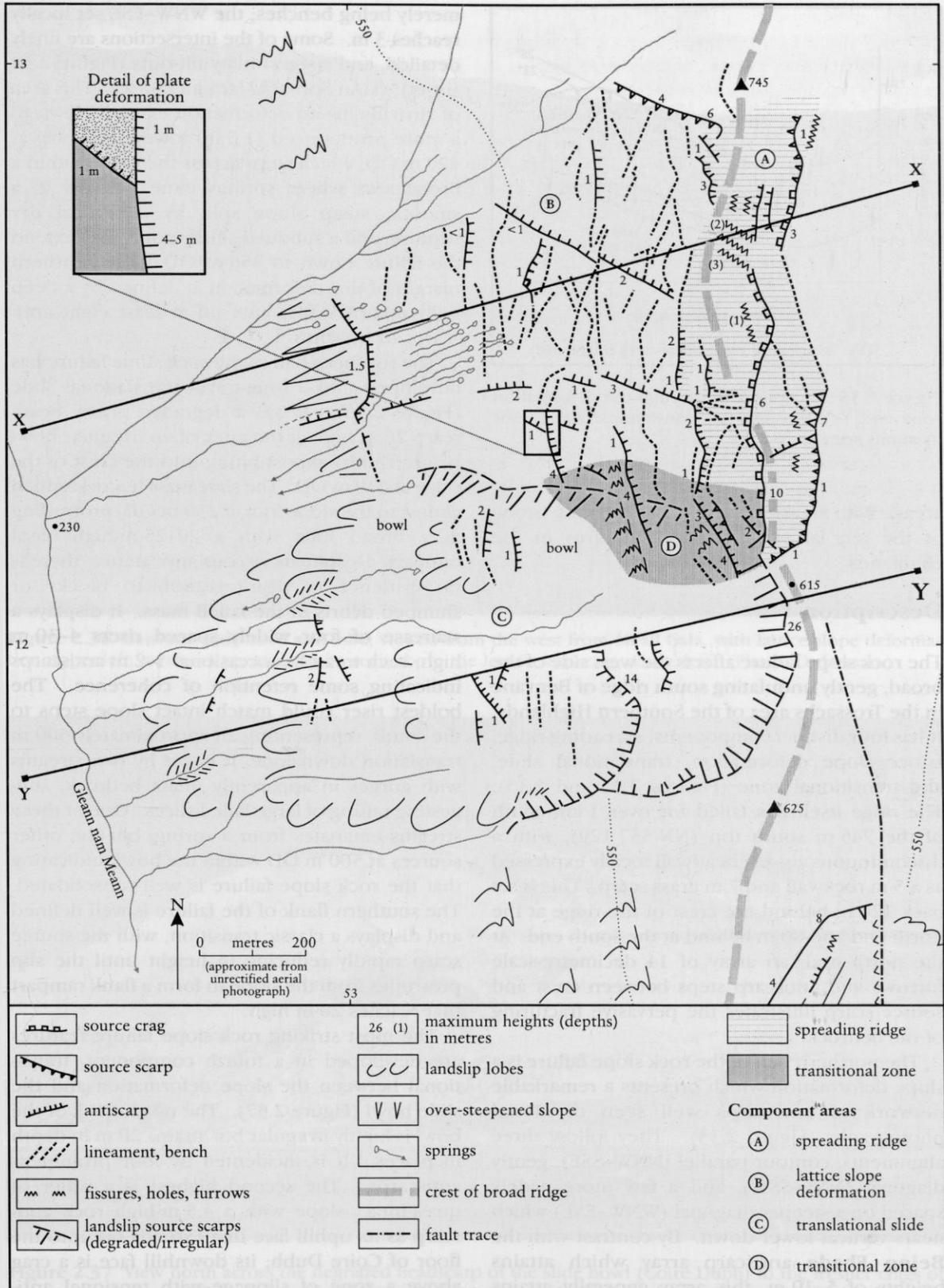
**Figure 2.34** Geomorphological interpretation of the Benvane rock slope failure complex. Based on unrectified aerial photograph with field verification.
