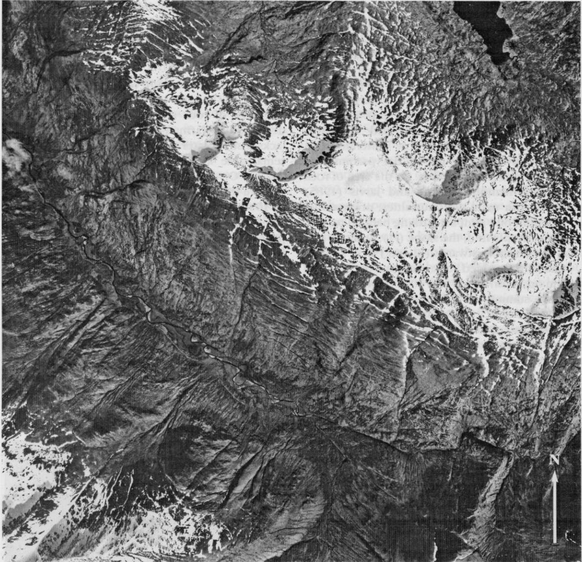
**Figure 2.20** Vertical aerial photograph of the Beinn Fhada rock slope deformation. The three major slope convexities are highlighted by anticarp arrays, as is the extent of the pre-glacial land surface with its structural lineaments. (Photo: Crown Copyright: RCAHMS (All Scotland Survey Collection).)
