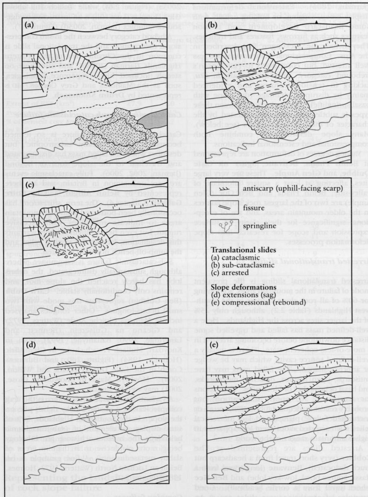
**Figure 2.5** Characteristic types of larger-scale rock slope failure identified in the Scottish Highlands. The plateau rim location is typical of less intensely dissected terrain. In more acute relief, headscarps may daylight below or behind the crest, or split the ridge. After Jarman (2006).
