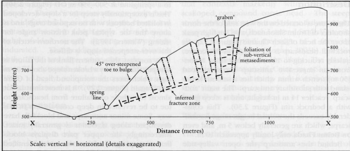
**Figure 2.30** Section X-X on Figure 2.29, showing over-steepened bulge and graben progressively tilting failed slices away from source. After Jarman (2003b).
