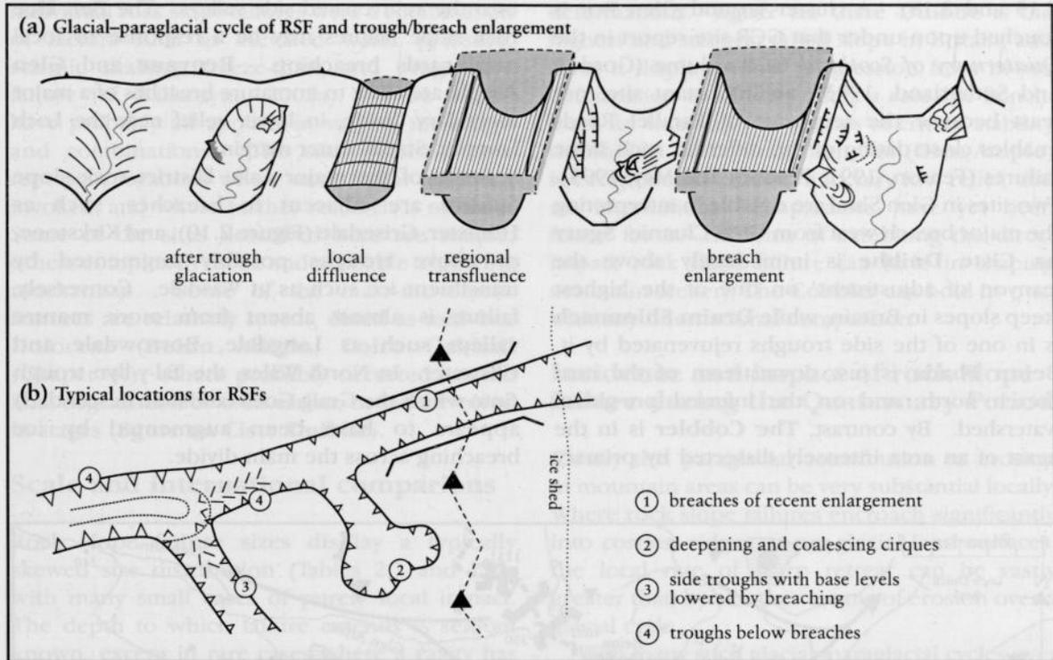
**Figure 2.16** (a) The inferred association of rock slope failure (RSF) with breach incision and enlargement over repeated glacial/paraglacial cycles. (b) Typical locations for rock slope failure responding to exceptional deglaciation stresses directly and indirectly associated with glacial breaching. After Jarman (2006).
