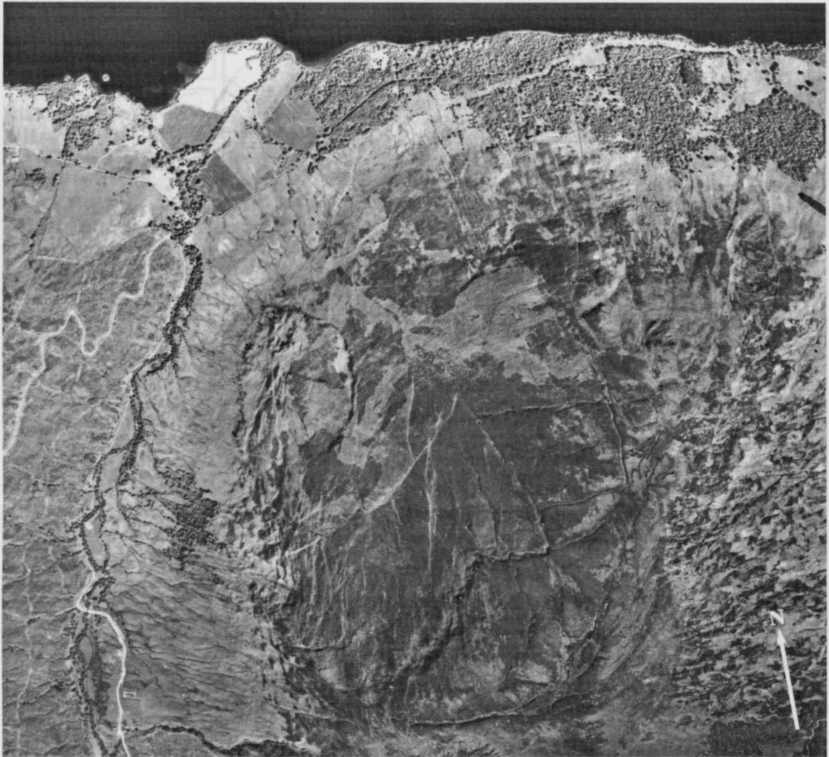
**Figure 2.41** Vertical aerial photograph (1989) of the Ben Our rock slope failure. (Photo: Crown Copyright: RCAHMS (All Scotland Survey Collection).)
