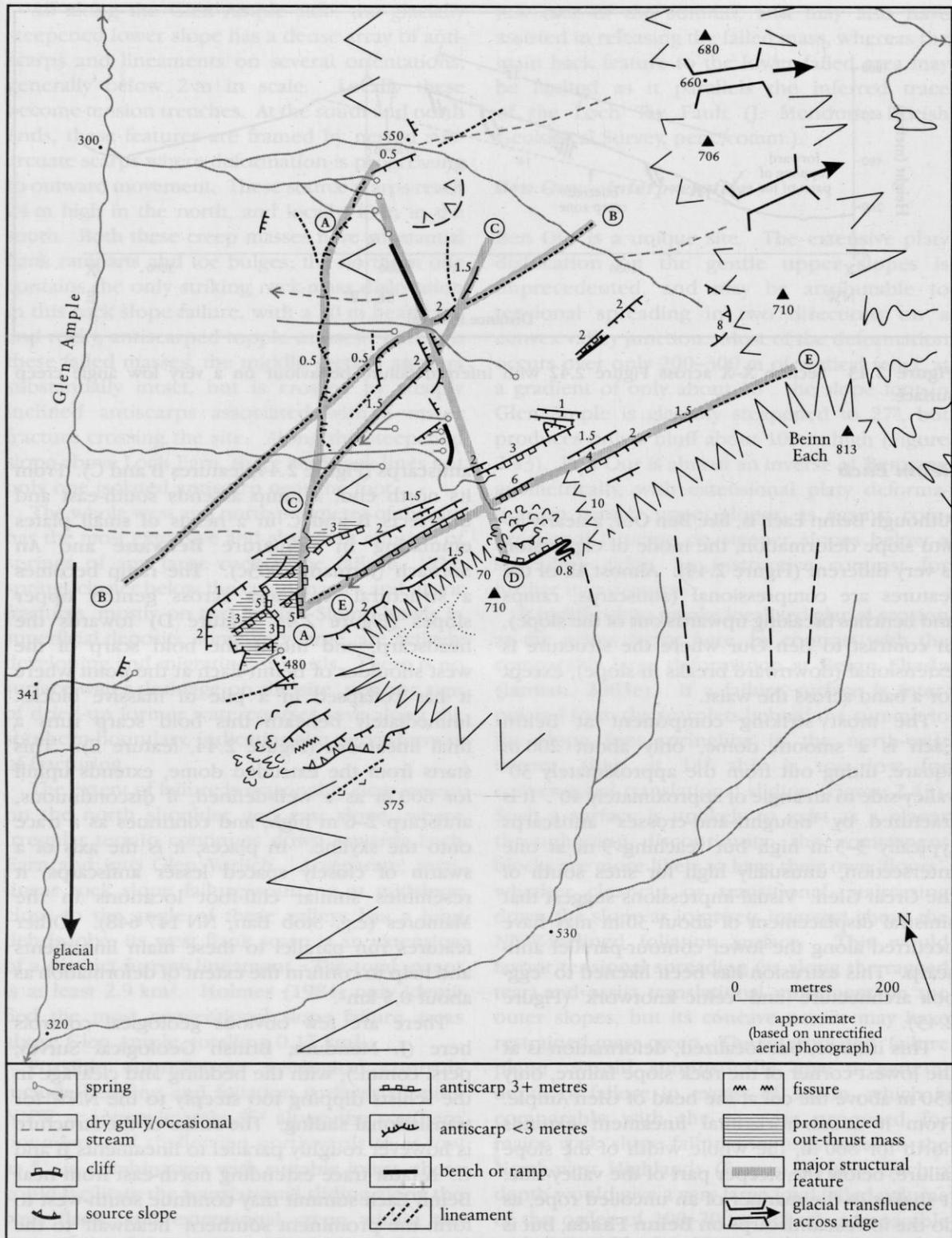
**Figure 2.44** Geomorphological interpretation of the Beinn Each rock slope failure. Features A, B, C, D and E are described in the text.
