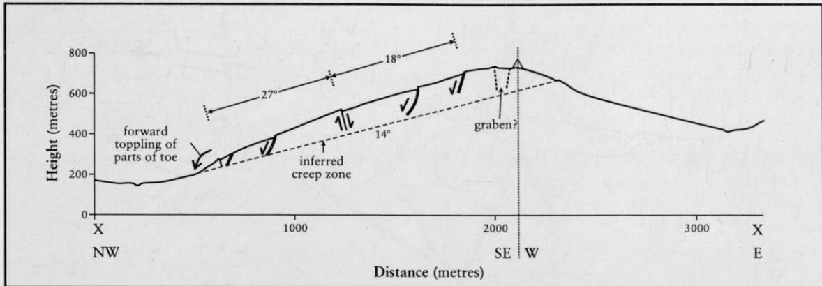
**Figure 2.43** Section X-X across Figure 2.42 with inferred failure behaviour on a very low angle creep surface.
