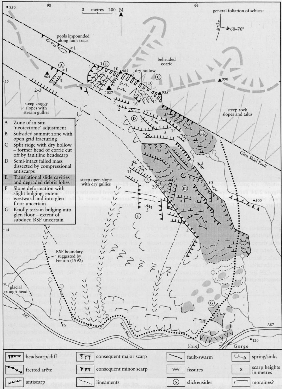
Figure 2.23 Geomorphological map of the Sgurr na Ciste Duibhe rock slope failure. After Jarman (2003b).
