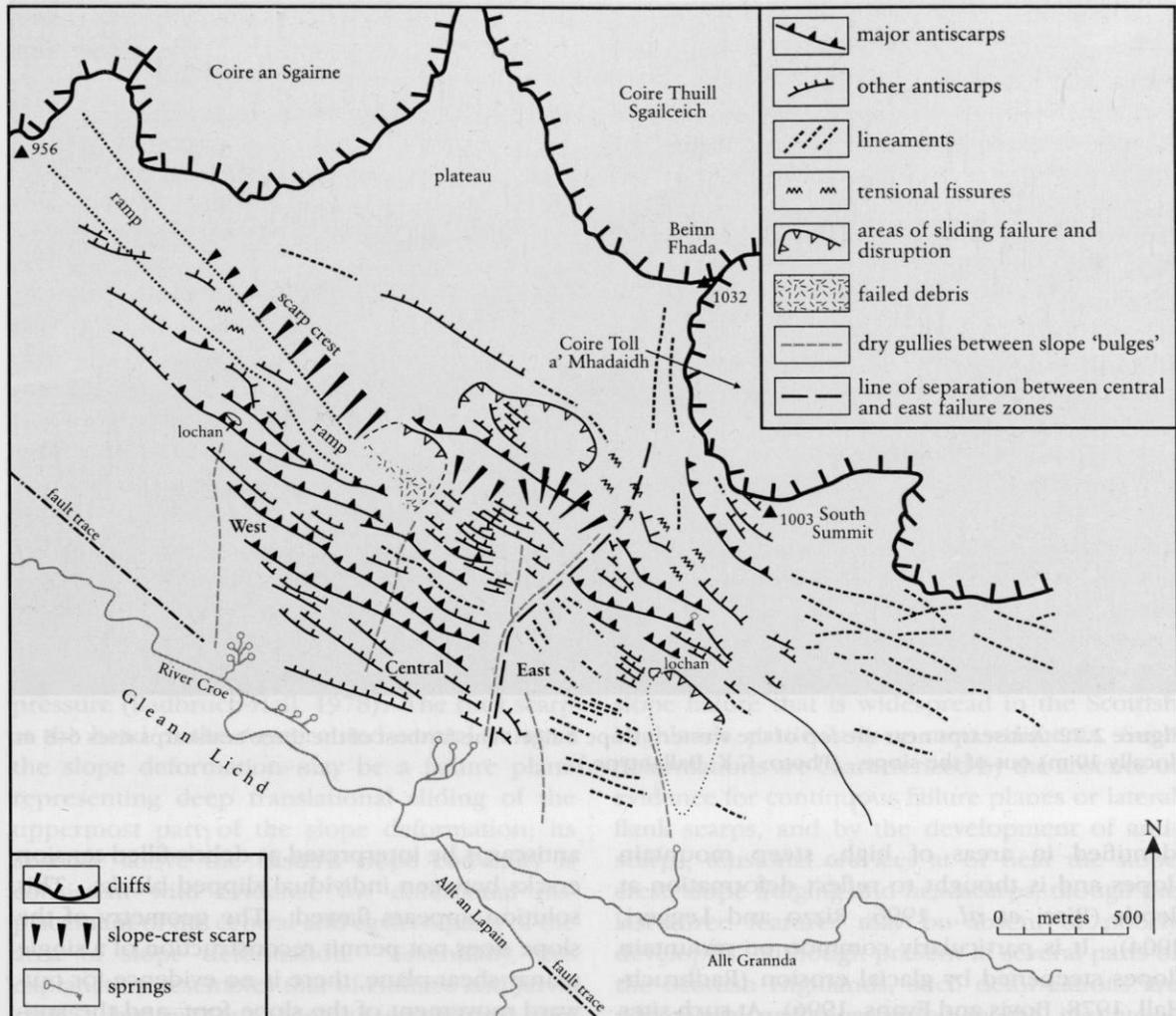
**Figure 2.21** Geomorphological map of the Beinn Fhada rock slope deformation, showing the location of prominent anticarps, lineaments, areas of localized sliding failure and the three slope convexities or bulges (labelled 'West', 'Central' and 'East'). The map is based on the aerial photograph in Figure 2.20, with an average scale of 1:22 500. After Jarman and Ballantyne (2002).
