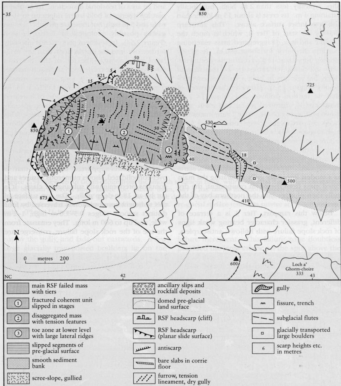
**Figure 2.52** Geomorphology of the Ben Hee rock slope failure (RSF) in An Gorm-choire. The encroachment into the undulating pre-glacial surface is considerably greater than the extent of the 'slipped segments'.
