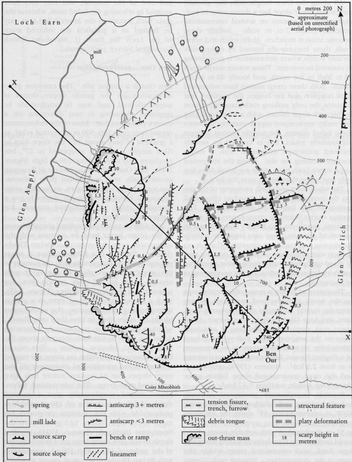
**Figure 2.42** Geomorphological interpretation of the Ben Our rock slope failure, based on the unrectified aerial photograph with field verification.
