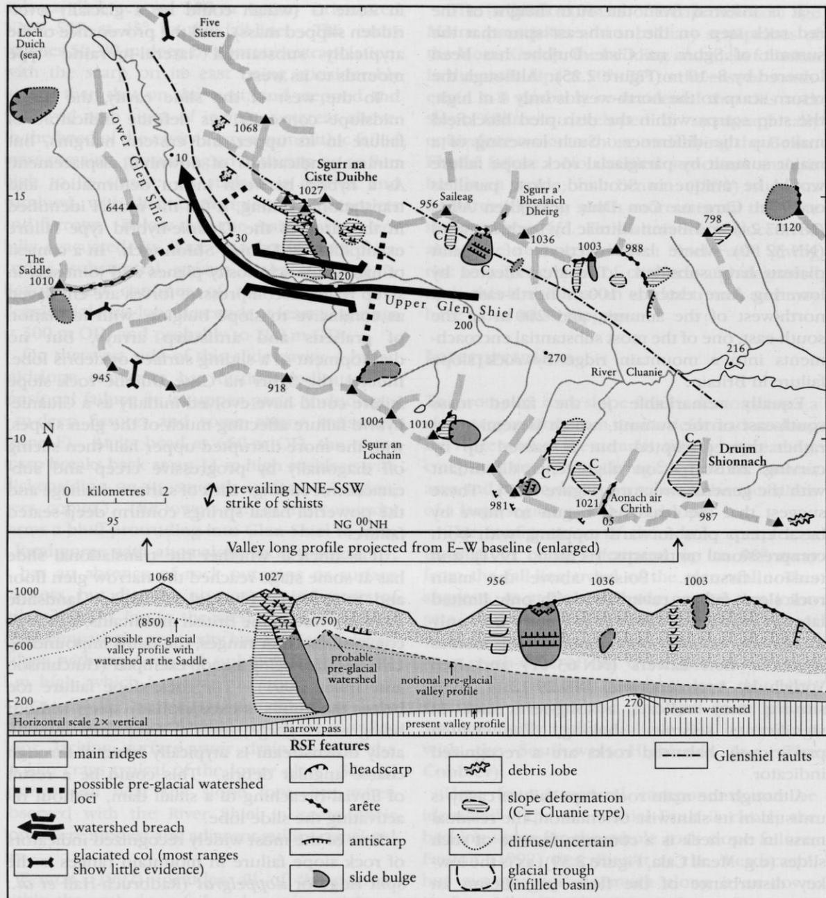
Figure 2.28 Map and long-section of the Glen Shiel breach with reconstructed pre-glacial watershed and associated rock slope failures on the north side of the main valley and in the trough corries of the south Cluanie ridge (e.g. Druim Shionnach). After Jarman (2003b).
