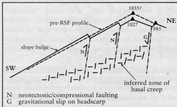
**Figure 2.25** Sgurr na Ciste Duibhe rock slope failure (RSF); notional cross-section of the summit area. After Jarman (2003b).
