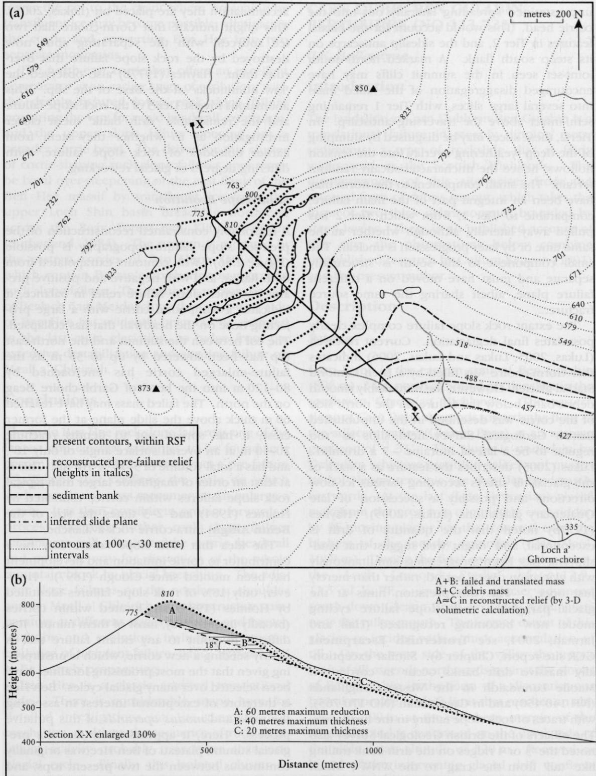
**Figure 2.56** The reconstructed pre-failure topography of An Gorm-choire, with the long-section of the main rock slope failure showing reduction of the summit ridge by up to 35 m and the scale of mass displacement.
