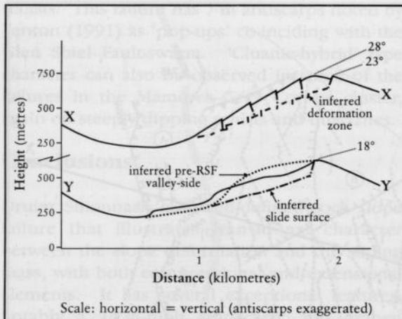
**Figure 2.35** Sections X–X through the deformation zone and Y–Y through the translational slide. For locations see Figure 2.34.
