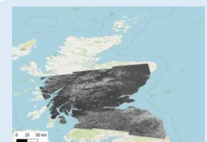
SEPA Illegal Waste Project coherence product example – darker pixels indicate low coherence and therefore change in elevation
