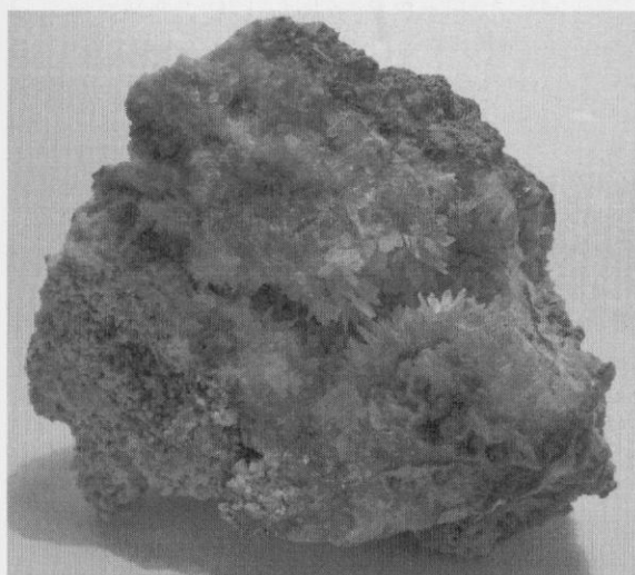
Figure 3.18 Specimen of crystallized barytocalcite from the spoil heaps adjacent to Foster's Hush. Sharply terminated monoclinic crystals project into vug in compact crystalline barytocalcite. The specimen is 80 mm across. (Photo: B. Young.)
