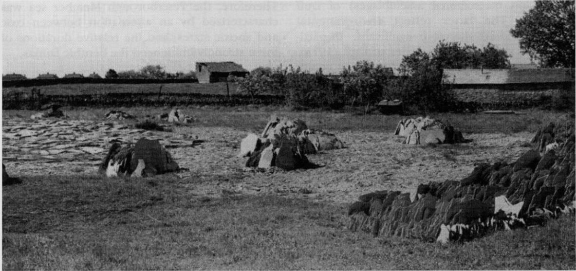
**Figure 4.28** Collyweston Slate workings showing slates stacked before trimming and slabs laid out for 'frosting'. (Photo: British Geological Survey, No. A8333, 1949.)
