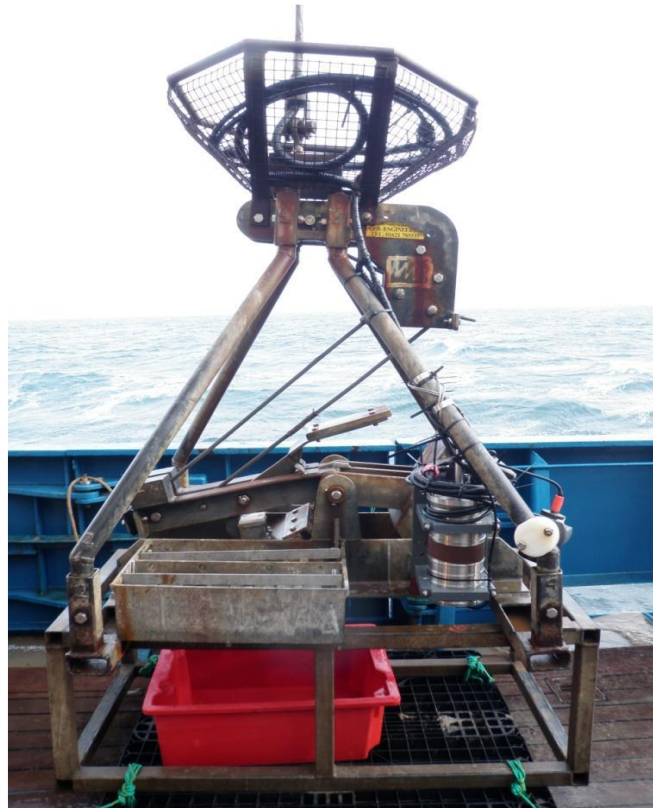
Figure 10. 0.1m 2 mini Hamon grab similar to that used on CEND0618.
