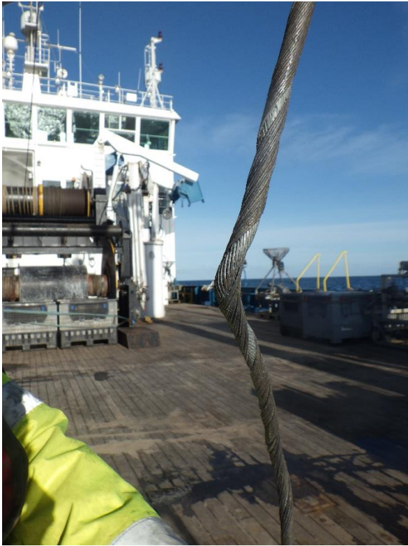
Figure 13. Damage to the camera sledge's fibre optic cable.
