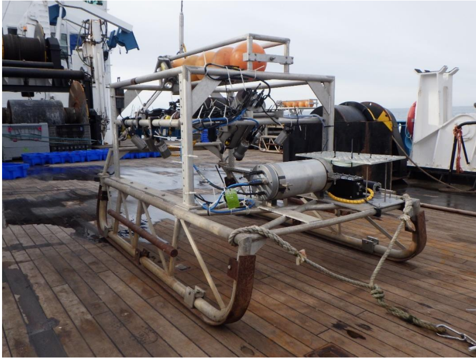
Figure 11. Camera sledge system used on CEND0618.
