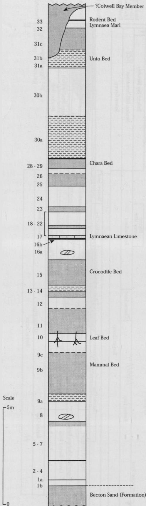
**Figure 6.15** A composite succession for the Totland Bay Member (Headon Hill Formation) at the eastern end of 'Barton Cliffs' (Hordle Cliff) (after Edwards and Daley, 1997). The bed numbers are those of Tawney and Keeping (1883).
