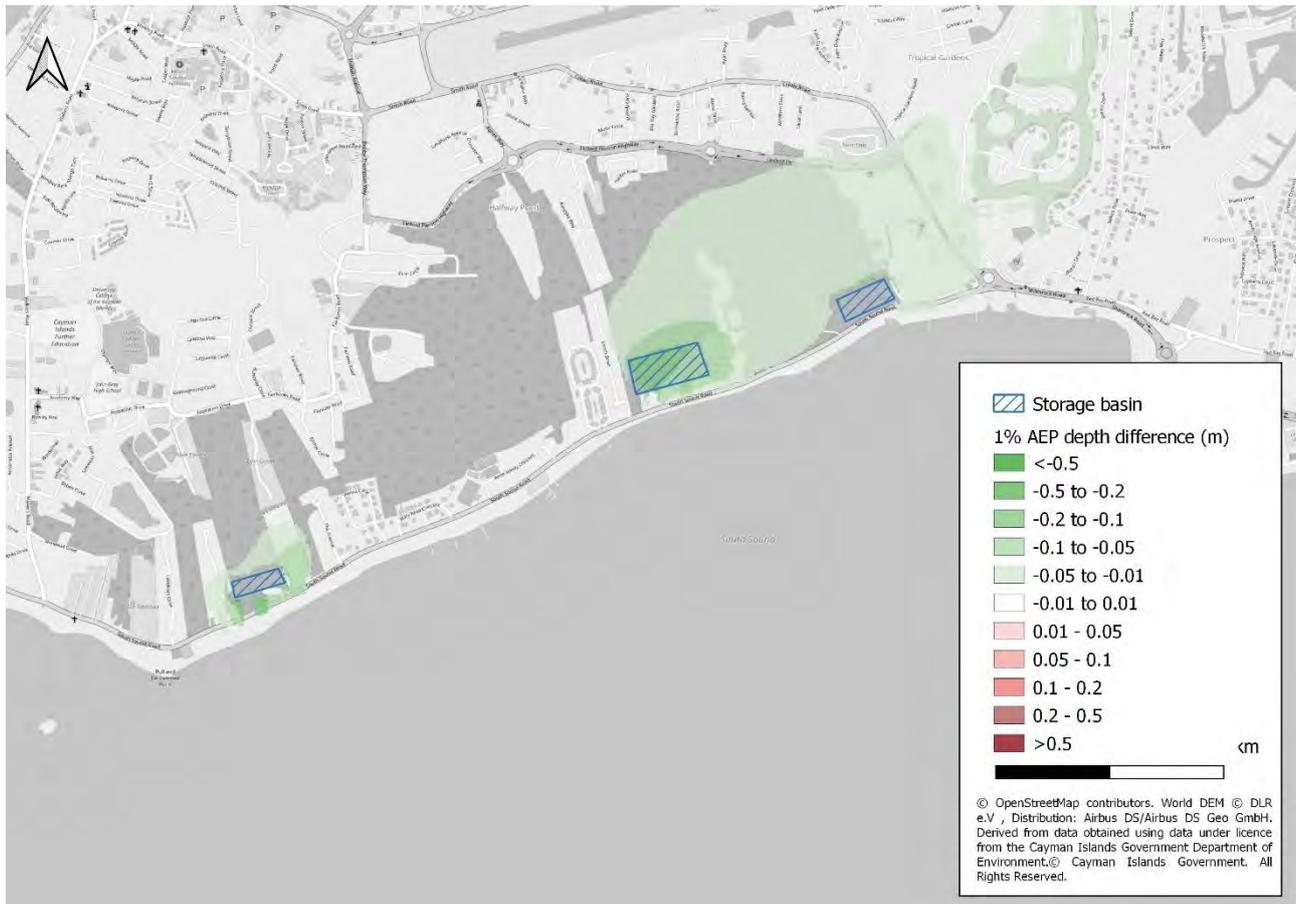
Typical depth reductions of 0.01-0.03m are anticipated within the eastern portion of the mangrove basin and adjacent canal network. More substantial reductions exceeding 0.10m are predicted in the local vicinity of each storage basin.
