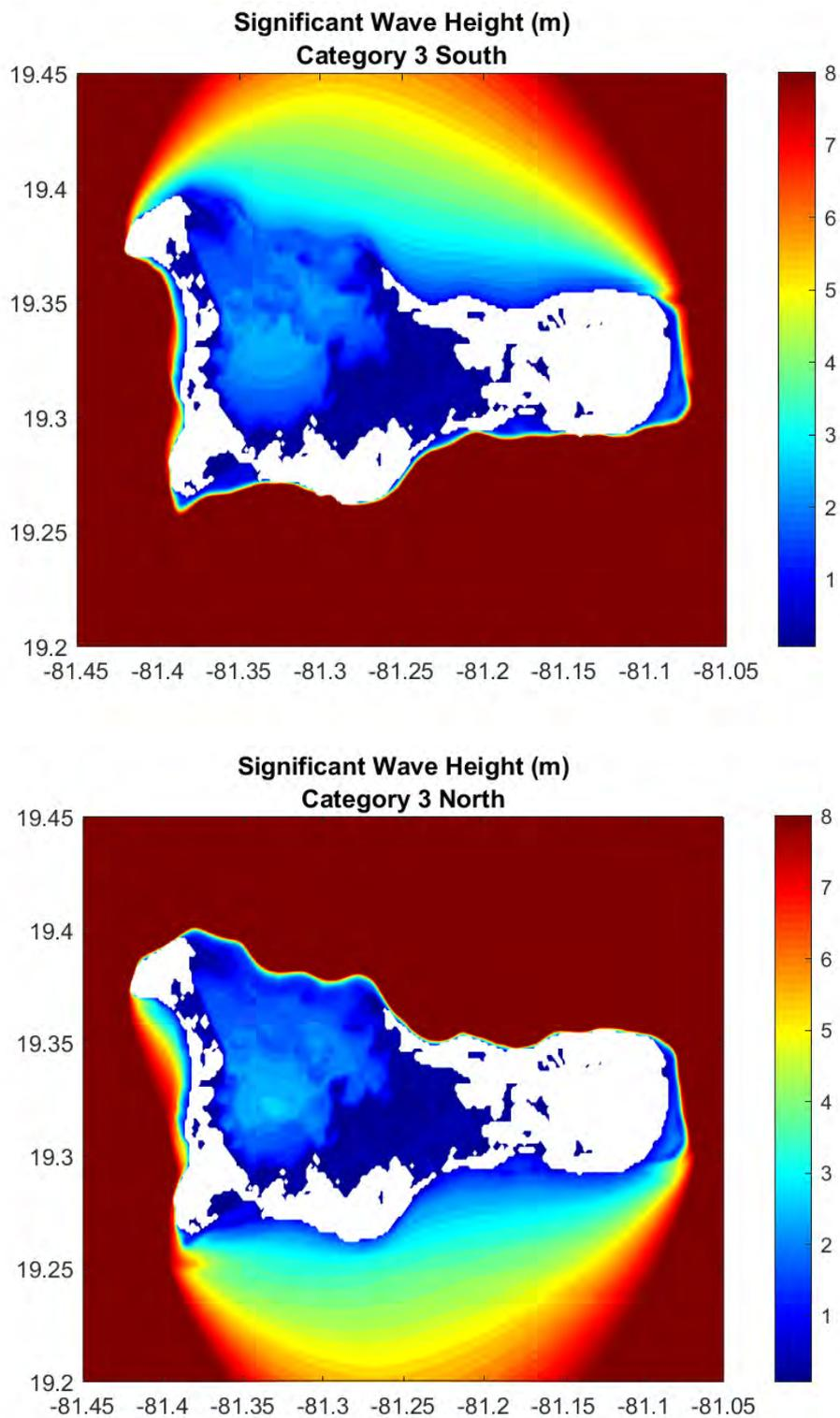
Figure 5.10 Significant wave height as modelled by SWAN with Category 1 hurricane winds from the south (top) and north (bottom).
