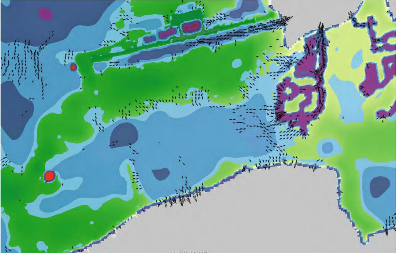
Note: Arrows show flow velocity and direction, indicating that water within the basin discharges to the South Sound Bay at several points to the south, and into the canal network to the east.
