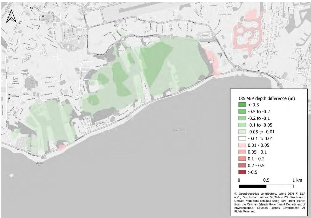
The enhanced scenario for South Sound assesses the impact of two potential storage basins that sit against the South Sound coastal road embankment. Additional drainage channel 'cuts' into the topography have been made to simulate the effects of drainage culverts to the sea. The 1% AEP event depth difference for this scenario is shown in Figure 5.6 below.
