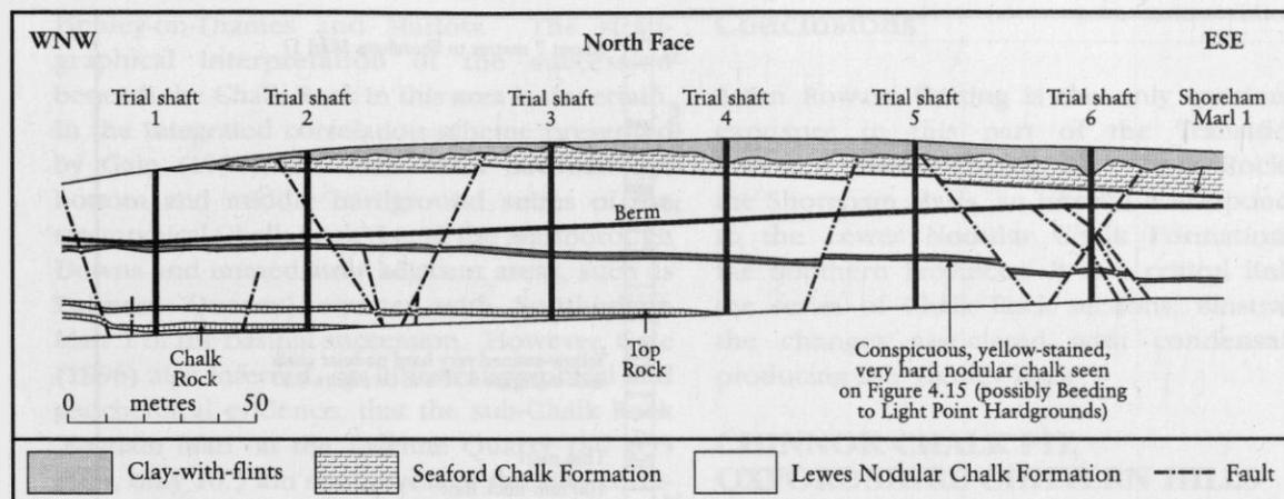
**Figure 4.17** Simplified geological section of the M40 Aston Rowant Cutting, Oxfordshire, constructed from field measurements and depths to marker beds in the original site investigation trial shafts.
