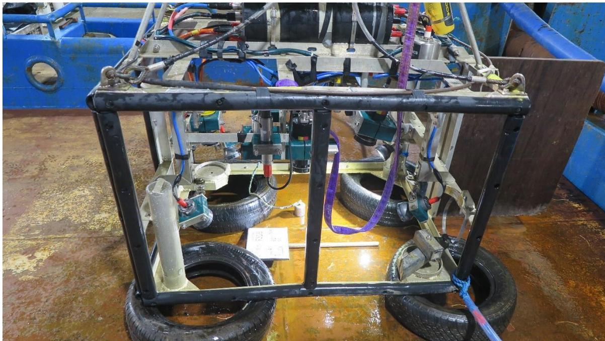
**Figure 10.** Drop-frame with video and still imaging system.
