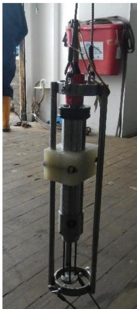
**Figure 13.** RBR Concerto<sup>3</sup> CTD with a Niskin water bottle and weight used on 1121S.
