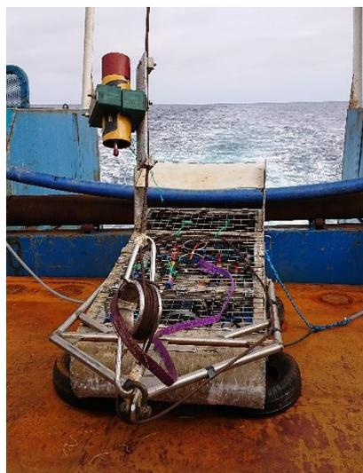
**Figure 11.** Towed camera chariot system used on 1121S.
