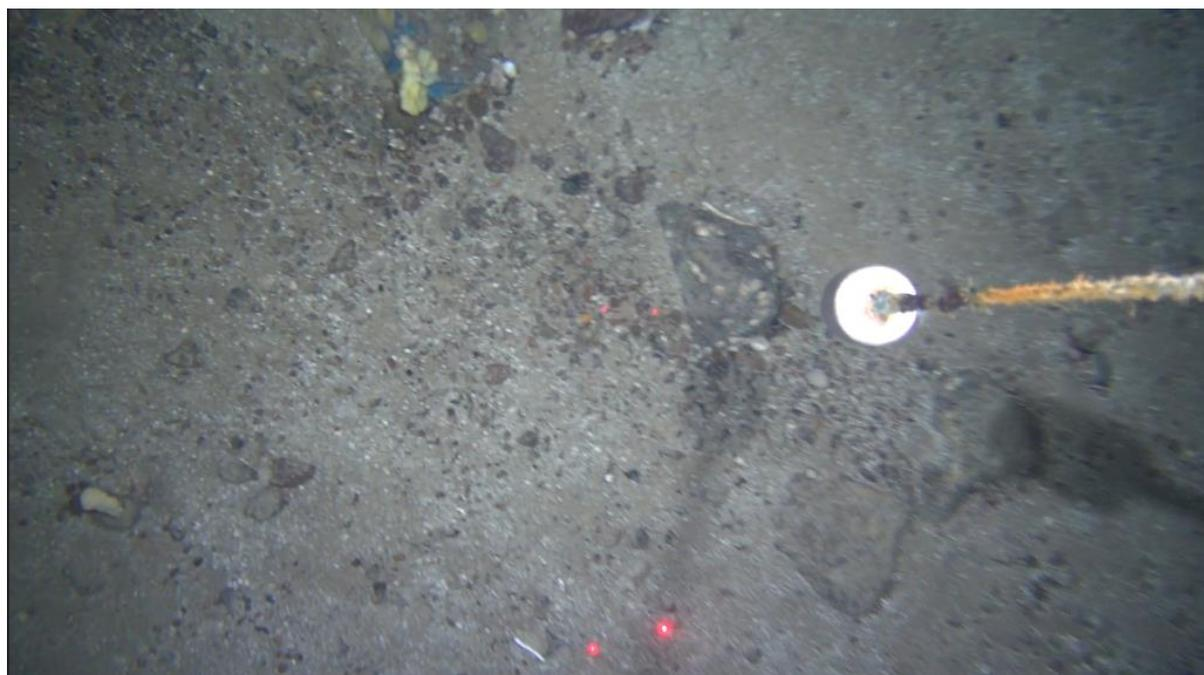
**Figure 11.** Video frame of laser scaling used on 1121S drop-frame. Red point lasers (centre) 64 mm spacing, note that these will not be visible on still images. Red point lasers (bottom) 120 mm spacing.
