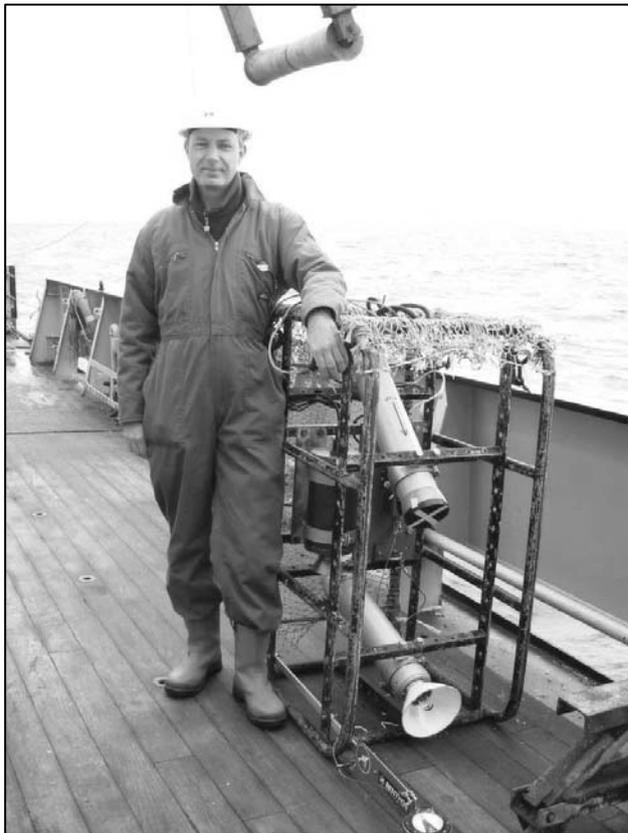
**Figure 2.1.** The "bed-hop" camera system in its supporting frame, just prior to deployment over the side of a research vessel.
