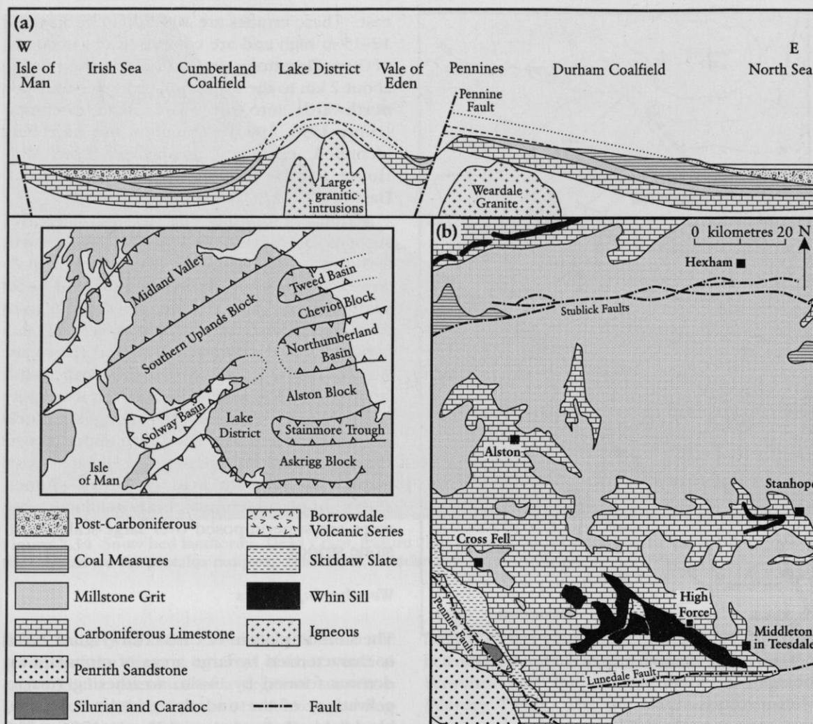
**Figure 7.36** (a) Regional geological section and main structural elements of northern England (after Taylor *et al.*, 1971). (b) Geological map of the central north Pennines (after Johnson and Hickling, 1970).
