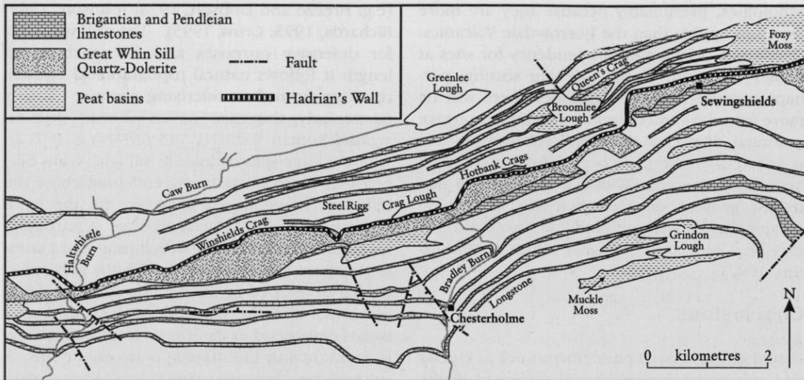
**Figure 5.71** Geological map of Hadrian's Wall in the vicinity of the Roman Wall GCR site (after Johnson, 1997). Note how the route of the wall follows the Whin Sill and the general ENE-WSW grain of the landscape.
