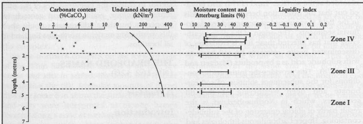
Figure 5.41 Weathering zones, carbonate content, undrained strength, moisture content, Atterberg limits and liquidity index versus depth in the lodgement till at Sandy Bay (after Eyles and Sladen, 1981).
