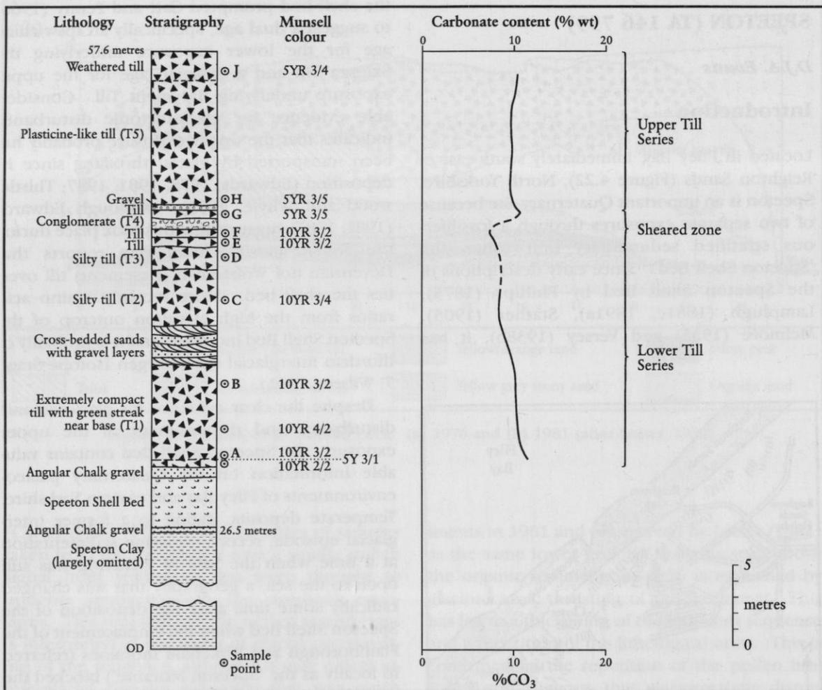
**Figure 4.23** Stratigraphical log of the complete Quaternary succession at New Closes Cliff (after Edwards, 1981), showing the relationship between the Speeton Shell Bed and the overlying Devensian Lower and Upper Till Series (Skipsea Till Formation, Evans *et al.*, 1995).
