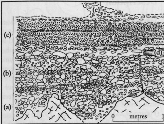
**Figure 4.19** Sedimentological detail of the Easington Raised Beach in the main exposure (after Bridgland and Austin, 1999). (a) Sand with cobbles, overlying uneven Magnesian Limestone surface; (b) well-bedded cobble and pebble gravel, with layers of fine shingle; (c) cemented gravel and pea-shingle; (d) cemented sand, current bedded; (e) unconsolidated gravel and shingle.
