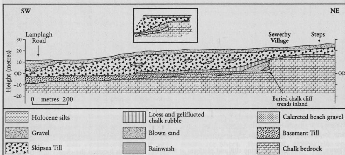
**Figure 4.28** The stratigraphical sequence at Sewerby based upon Lamplugh (1887) and Catt (1987c). An alternative stratigraphical relationship between the Basement Till and the interglacial beach gravels based upon Lamplugh (1890) and most recently preferred by Eyles *et al.* (1994) is reproduced in the inset.
