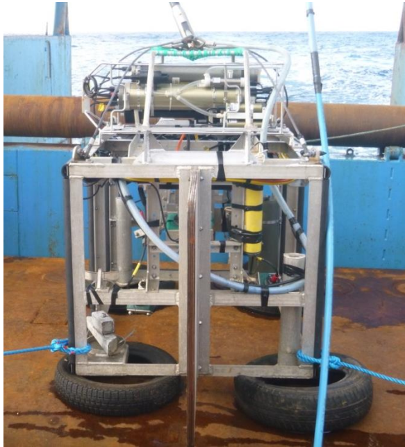
Figure 2: Drop-down video camera frame used on 1512S survey.
