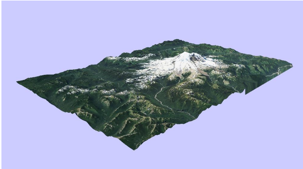
Figure 5. 3D model of United States Geological Service DEM and imagery for Mount Rainier (Information on More 3D Maps and Tips using QGIS2ThreeJS ).
