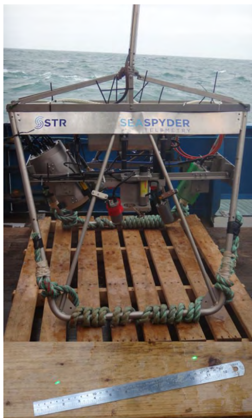
Figure 5. The drop frame mounted high definition camera and laser scaling (220mm linear maximum).
