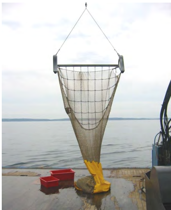
Figure 6. Recovery of the scientific (Jennings) 2m beam trawl on the back deck of the RV Cefas Endeavour.
