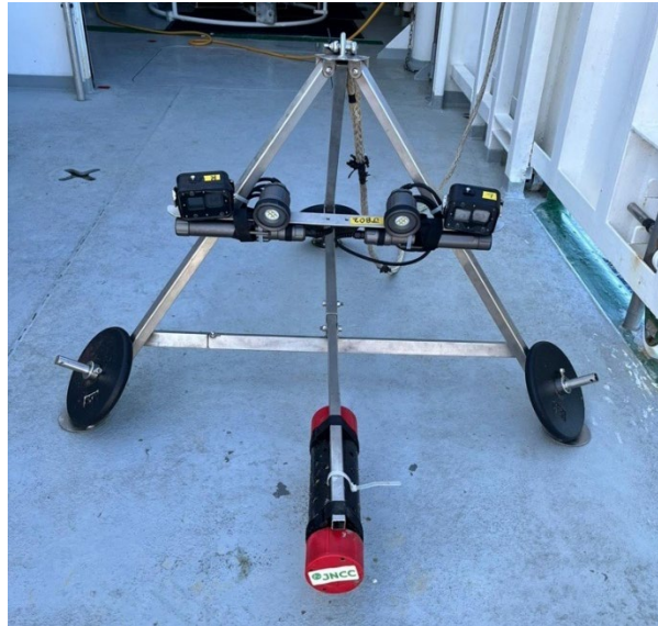
Figure 11. BRUV camera system used on the TC25023 survey of North-West of Jones Bank MPA.
