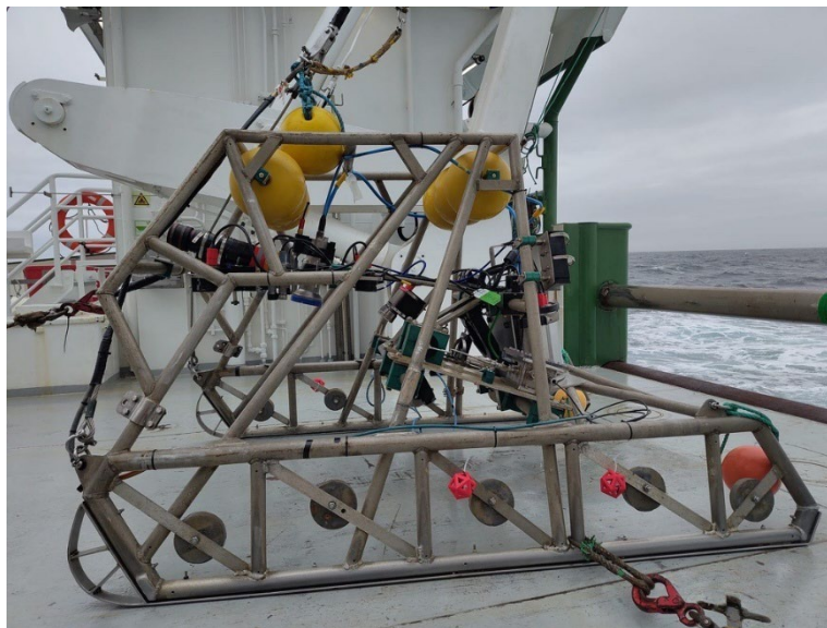
Figure 10. The Marine Institutes camera sledge system. eDNA metaprobes are attached to cross braces on the sledge runners.
