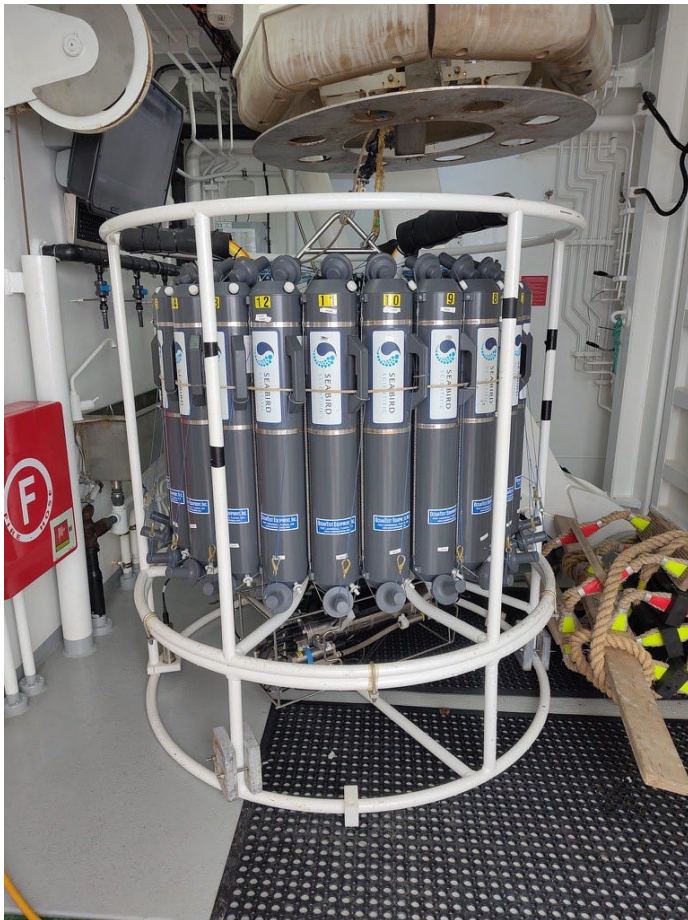
Figure 12. CTD rosette and Niskin bottles used on the TC25023 survey of North-West of Jones Bank MPA.
