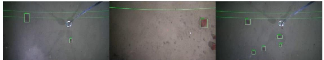
Figure 14: Sea pen detections in Video S using the RFCN model. Detections from this CNN are shown as green boxes. The white boxes are from the DeepSORT tracking algorithm. The green number refers to the DeepSORT identification given to the tracked instance and does not necessarily reflect the count of instances.
