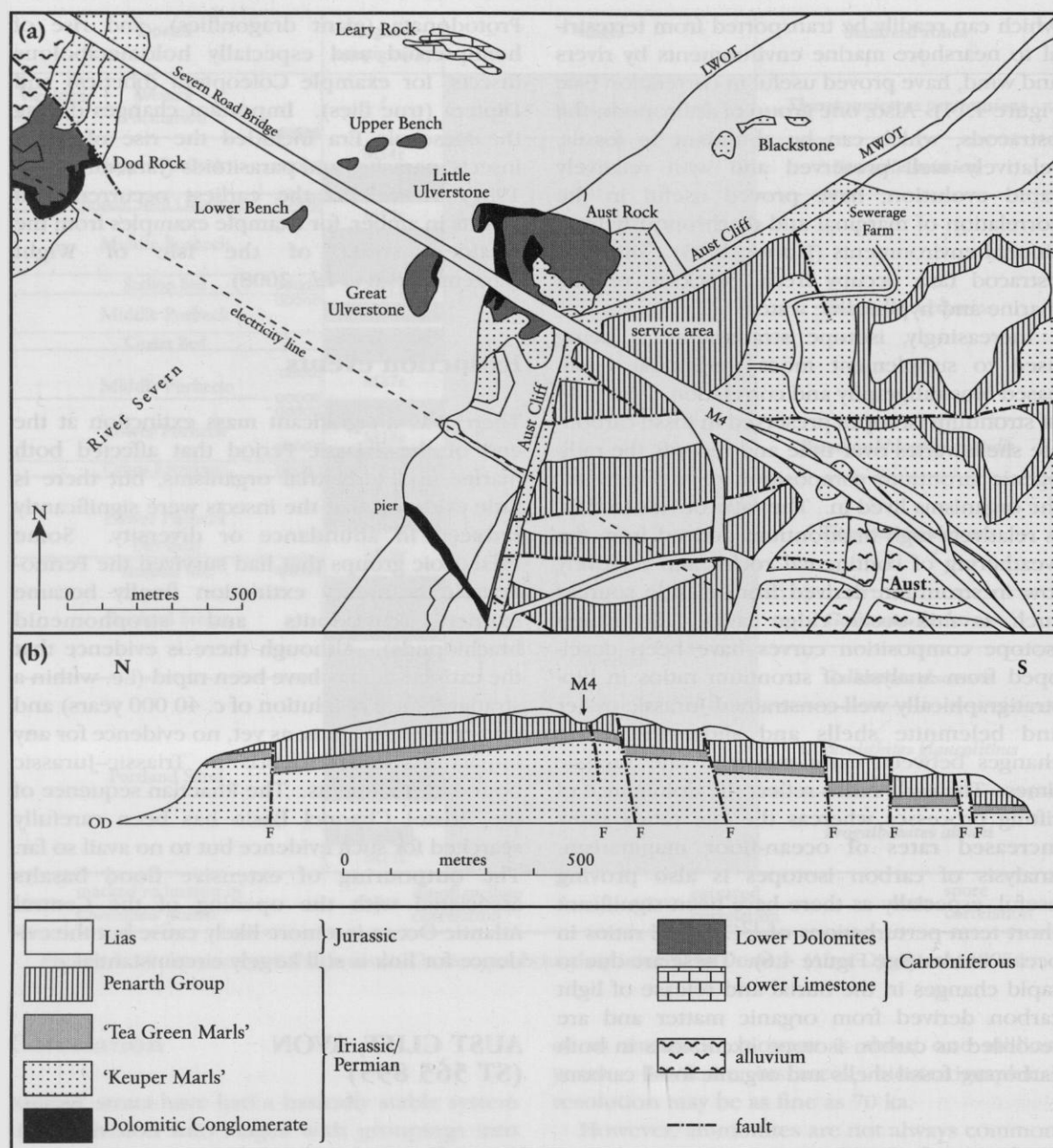
Figure 4.15 Triassic and Jurassic strata at Aust Cliff (a) geological map, and (b) the broad anticlinal structure. (After Hamilton, 1977.)
