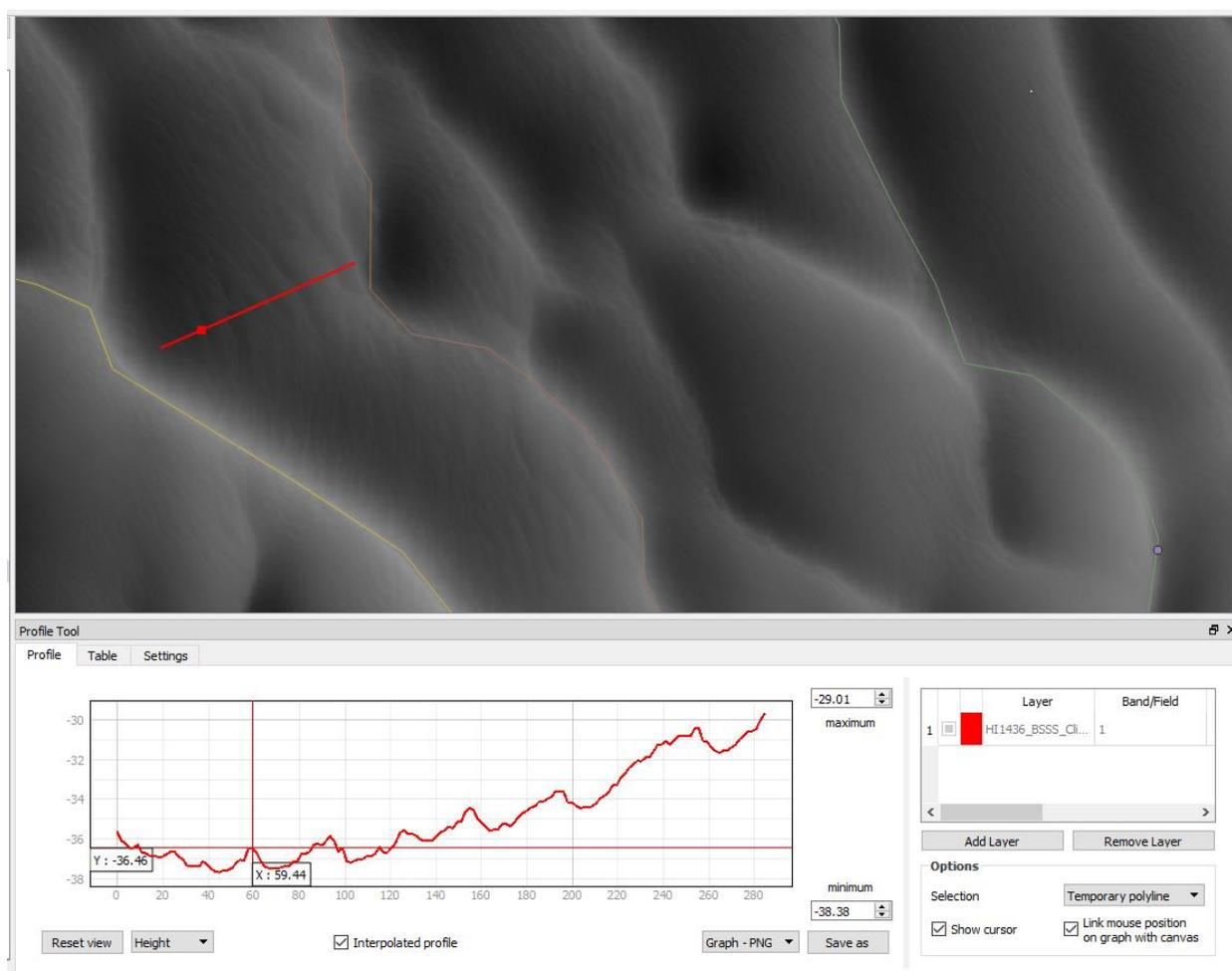
**Figure 7.** Fine-scale topography profiles of sandwaves associated with the megaripple field on the NW flank of the sandbank feature based on multibeam echosounder (MBES) data collected within the Bassurelle Sandbank SAC in 2014.
