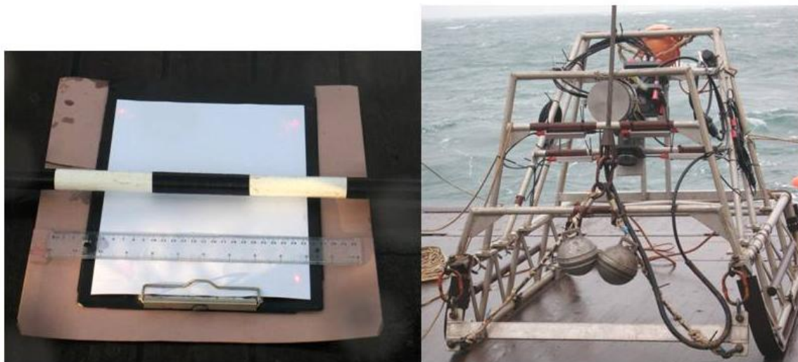
Figure 5. Sledge mounted camera system and scaling lasers used to determine field of view and size.
