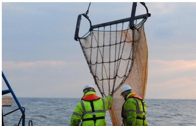
Figure 4. 2m Jennings beam trawl used to collect epibenthic specimens.
