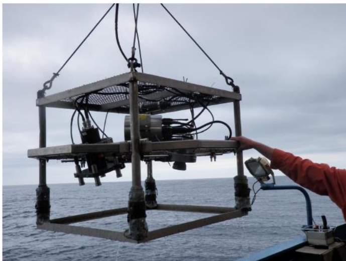
Figure 6. Drop camera frame fitted with video and still imaging system.
