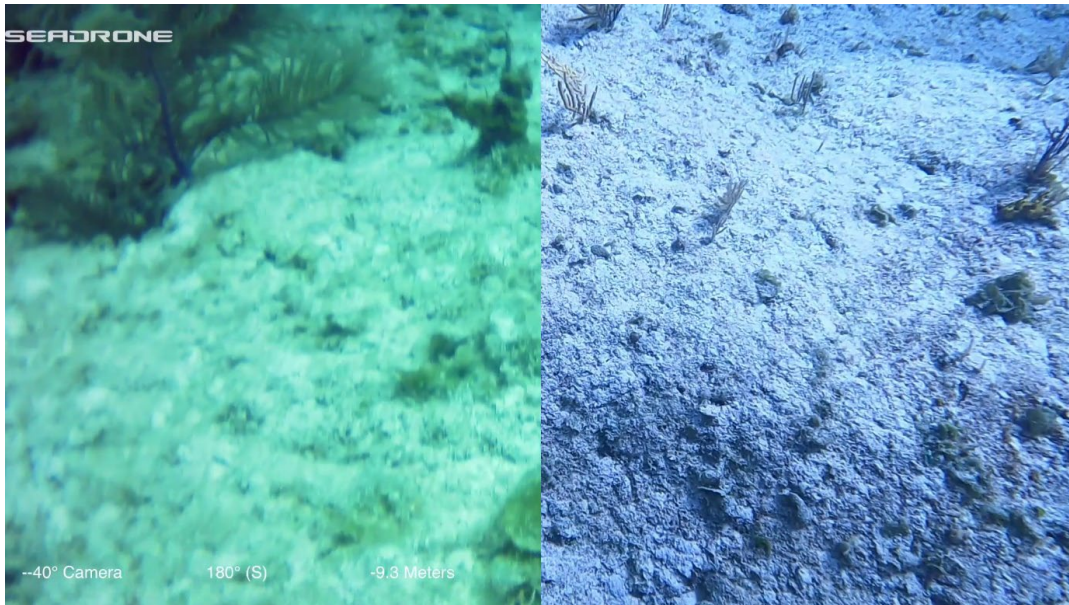
Figure 6. Comparison of video stills from the Seadrone (left) and the GoPro on the TVM (right), taken at a comparable depth and conditions
