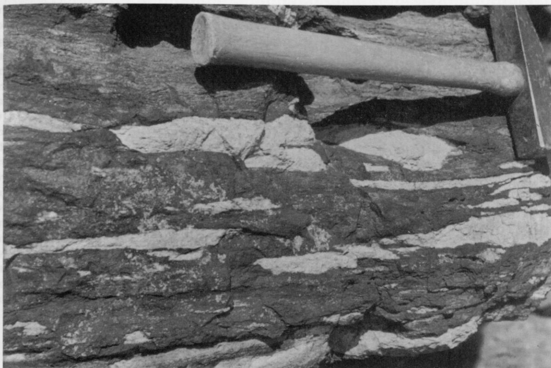
Figure 4.22 Typical, banded, basic hornfels of volcanic origin, composed of dark layers of hornblende and biotite, with light-coloured, segregation lenses of diopside. Tater-du, Cornwall. (Photo: P.A. Floyd.)
