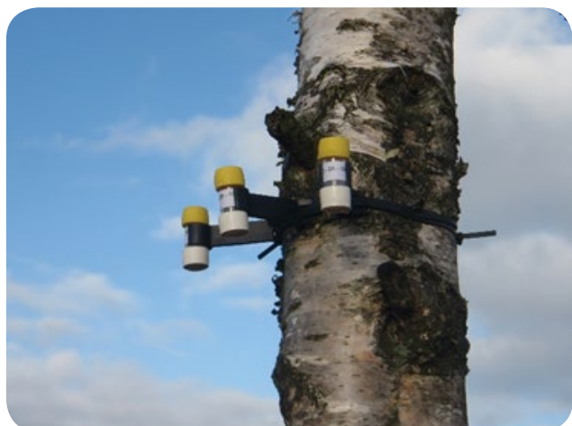
Passive Sampling of Ammonia on a Special Area of Conservation © JNCC/Clare Whitfield
