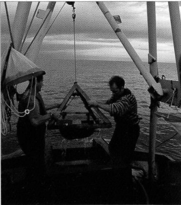
Remote sampling by grab is used to sample biotopes over extensive areas of sediment. Northumberland coast (Aquatic Environmental Services/JNCC).
