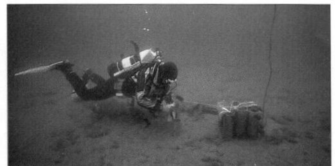
During diving-based surveys or in areas where sediments are restricted in distribution, coring by divers, together with digging over the sediment for large widely dispersed species is used to record from sublittoral sediment biotopes. Ceredigion coast (Paul Brazier/JNCC).
