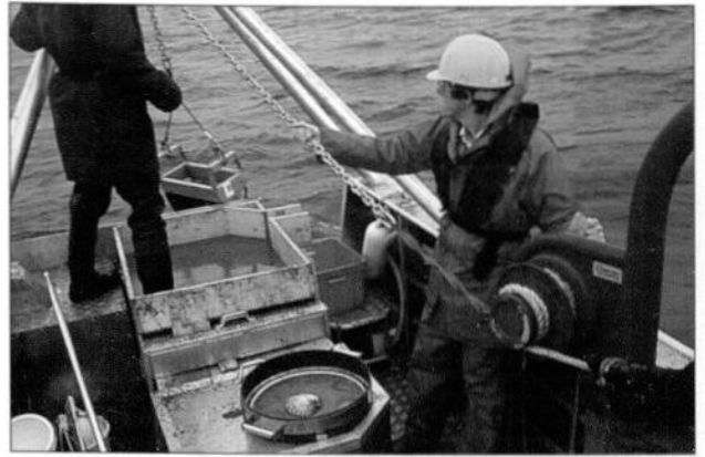
The MNCR launch Swiftia can be used to sample sediments using a dredge (Keith Hiscock/JNCC).
