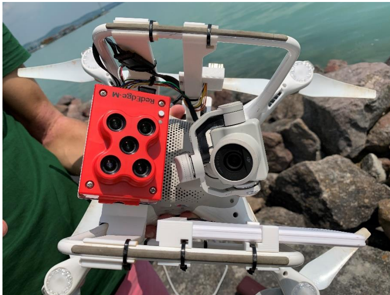
Micasense RedEdge payload added to DJI drone Using 3D-printable mounts
