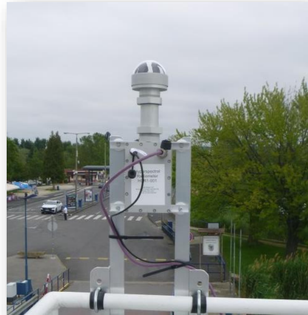
Peak Design HSR-1 diffuse/direct irradiance (replacing robotic sun-photometer)
