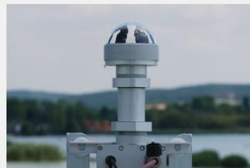
Hyperspectral Radiometer for Global & Diffuse Irradiance (HSR1)
