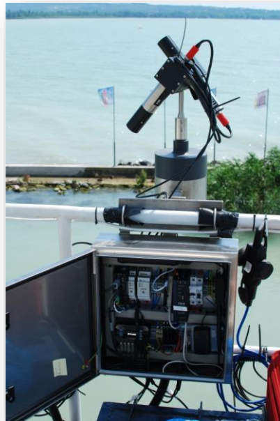
PML Solar-tracking Radiometry platform (moving platforms, use existing sensors, open- source approach)
