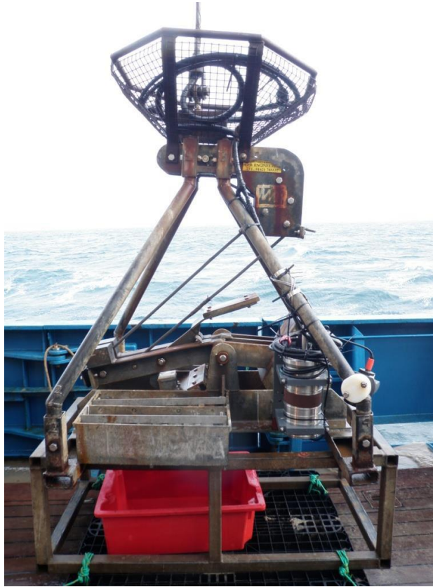
Figure 5. Mini Hamon grab with video camera (Ham Cam).
