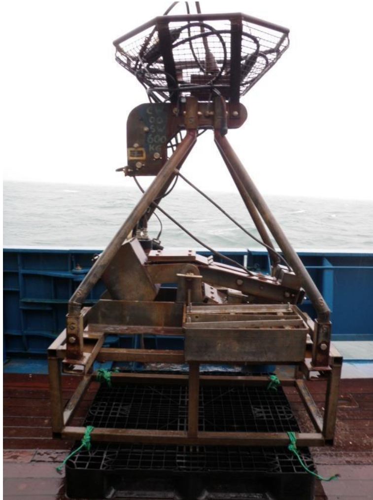
Figure 2. Mini Hamon grab with video camera (HamCam).
