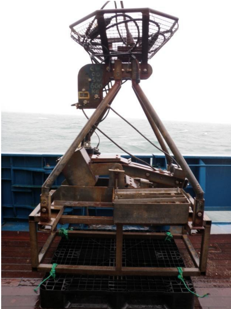
Figure 4. Mini Hamon grab with video camera (HamCam).
