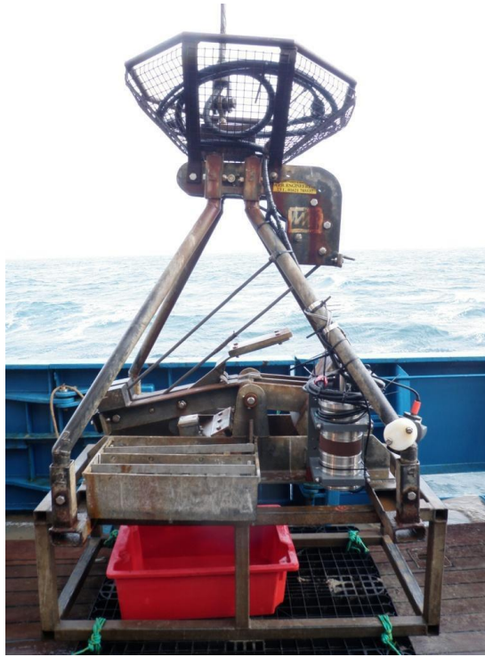
Figure 3. 0.1m 2 mini Hamon grab with video camera.
