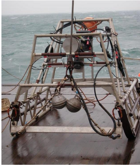
Figure 3. Camera sledge with video and still imaging system.
