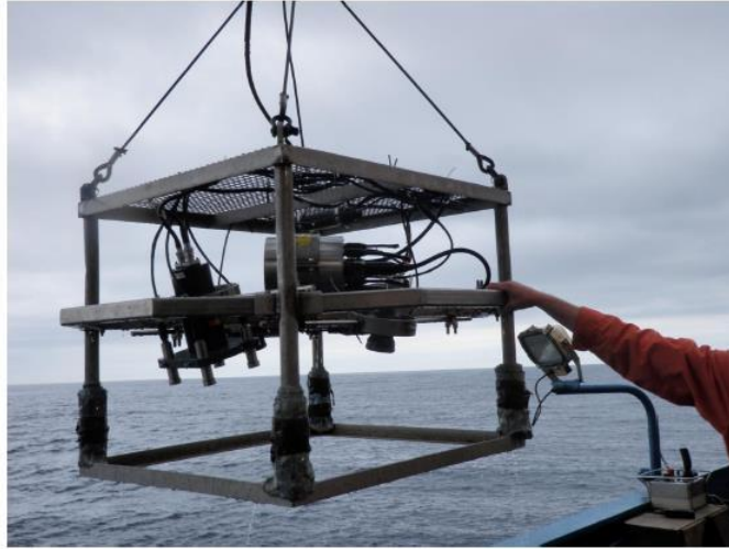
Figure 4. Drop camera frame fitted with video and still imaging system.
