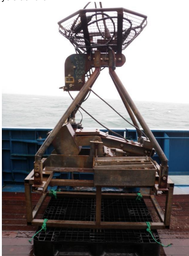
Figure 3. Mini Hamon grab with video camera (HamCam).
