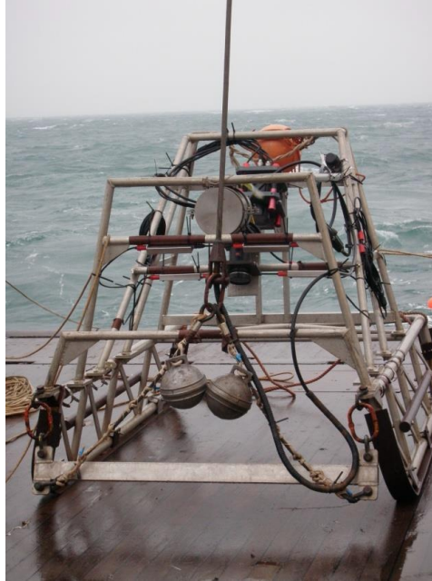
Figure 4. Camera sledge with video and still imaging system.
