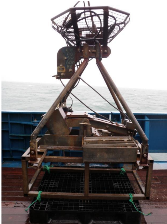
Figure 2. Mini hamon grab with video camera (HamCam).
