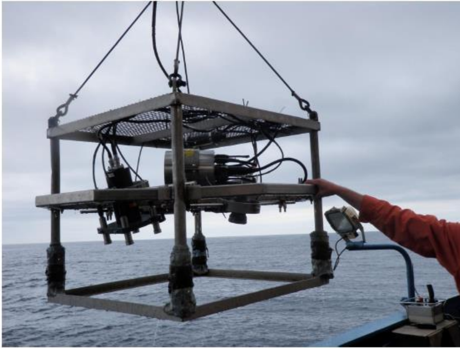
Figure 5. Drop camera frame fitted with video and still imaging system
