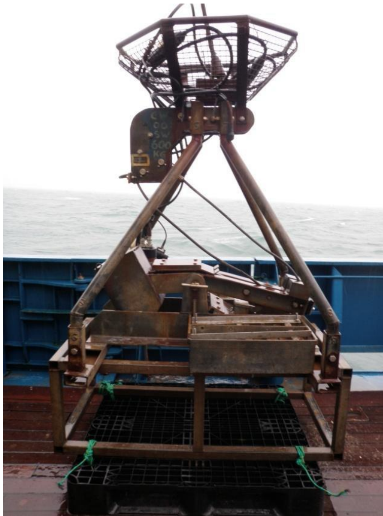
Figure 2. Mini Hamon grab with video camera (HamCam).
